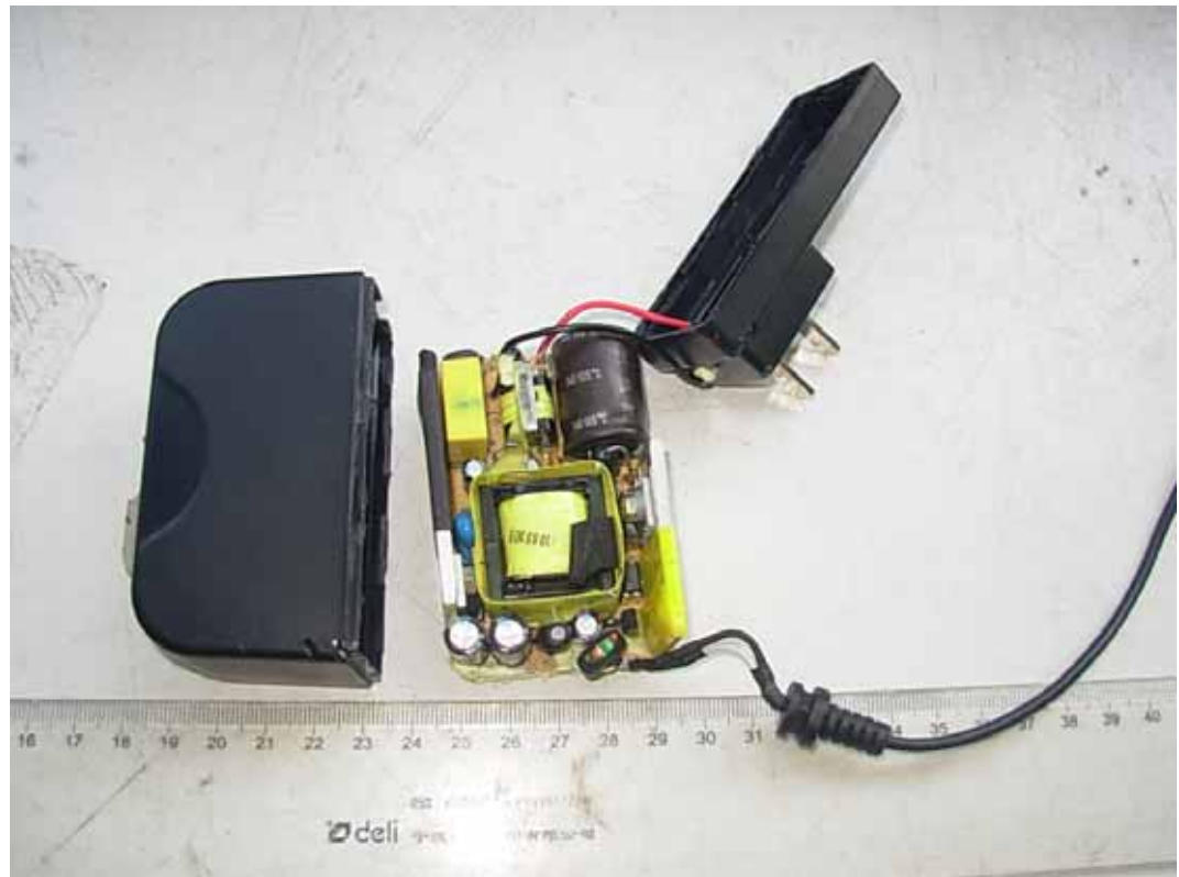
FIGURE 9 LCD MONITOR (M/N: E1948SX) ADAPTOR (COVER REMOVED)
