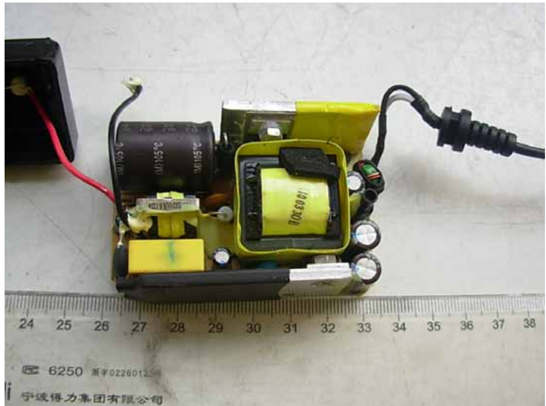
FIGURE 10 LCD MONITOR (M/N: E1948SX) ADAPTOR (MAIN BOARD – COMPONENT SIDE)
