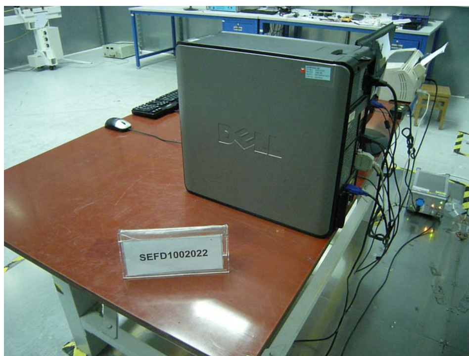
Back View of Conducted Emission Test
