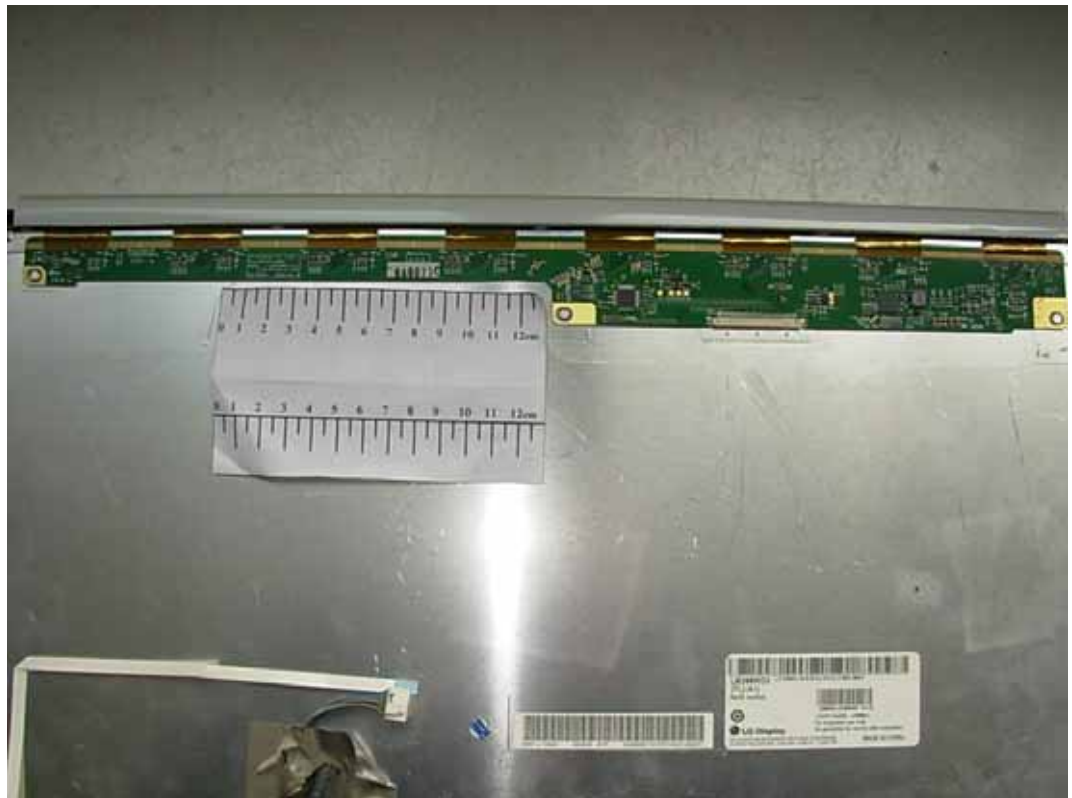
FIGURE 8 LCD MONITOR (M/N: E2050SV) LCD PANEL MAIN BOARD (COMPONENT SIDE)
