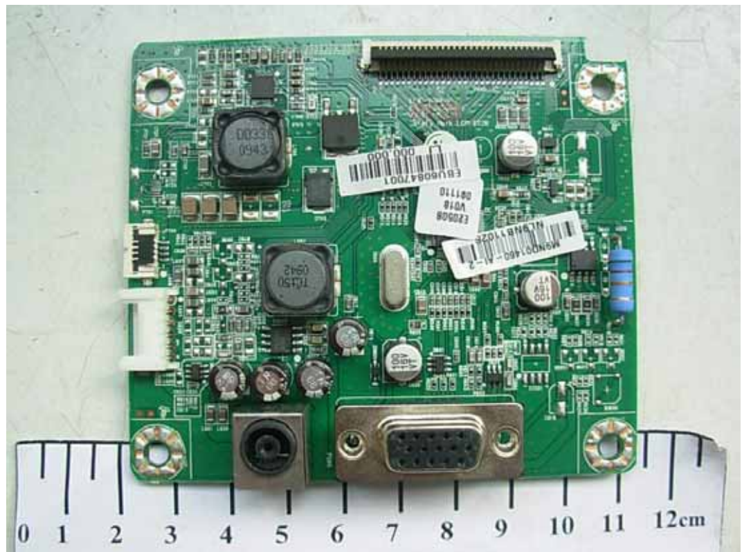
FIGURE 2 LCD MONITOR (M/N: E2050SV) MAIN BOARD (COMPONENT SIDE)
