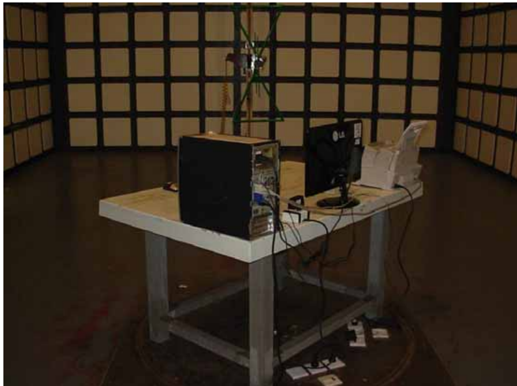
SETUP WITH MAXIMUM DETECTED EMISSION AT VERTICAL POLARIZATION (TEST MODE: D-SUB 640*480@60Hz) (ADAPTER: ADS-24S-12 1224GPG)
