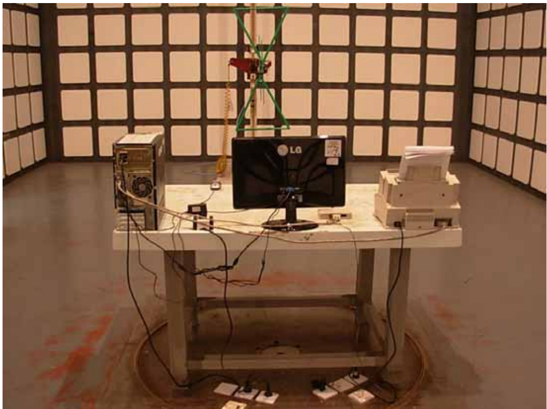
BACK VIEW OF RADIATED EMISSION TEST
