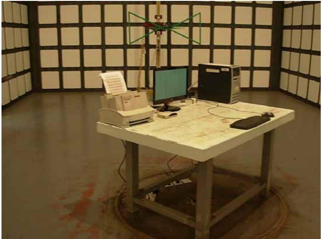
SETUP WITH MAXIMUM DETECTED EMISSION AT HORIZONTAL POLARIZATION (TEST MODE: D-SUB 640*480@60Hz) (ADAPTER: ADS-24S-12 1224GPG)
