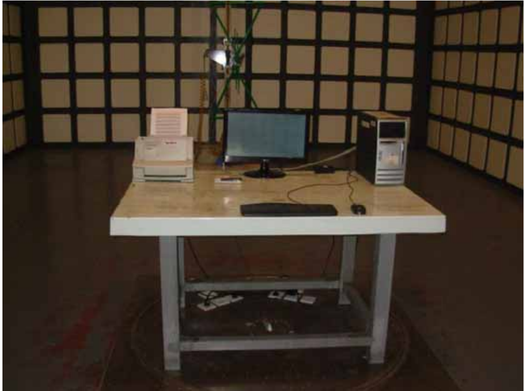
FRONT VIEW OF RADIATED EMISSION TEST
