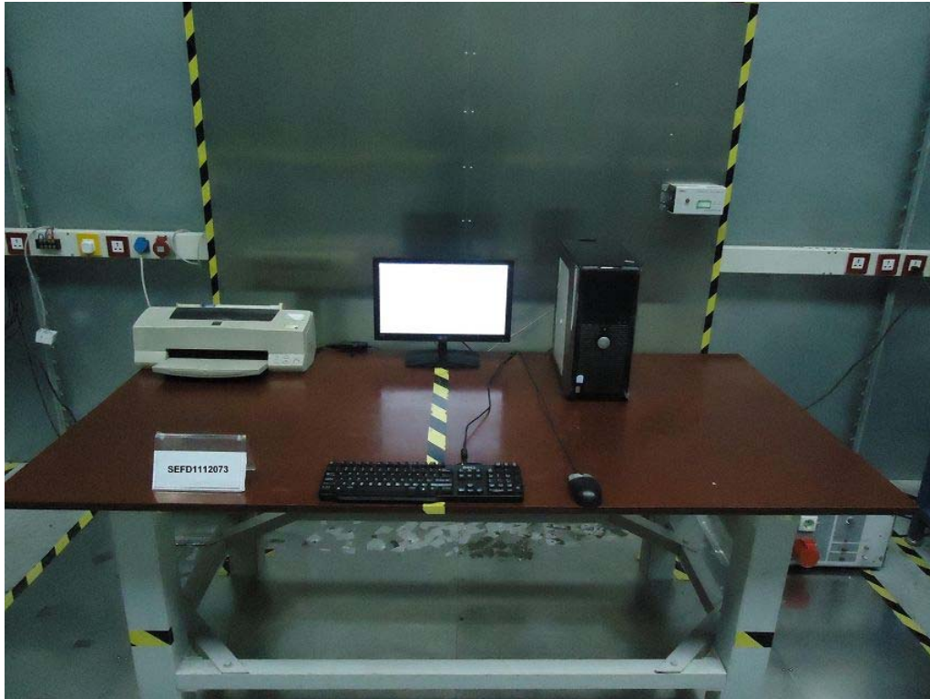
Front View of Conducted Emission Test
