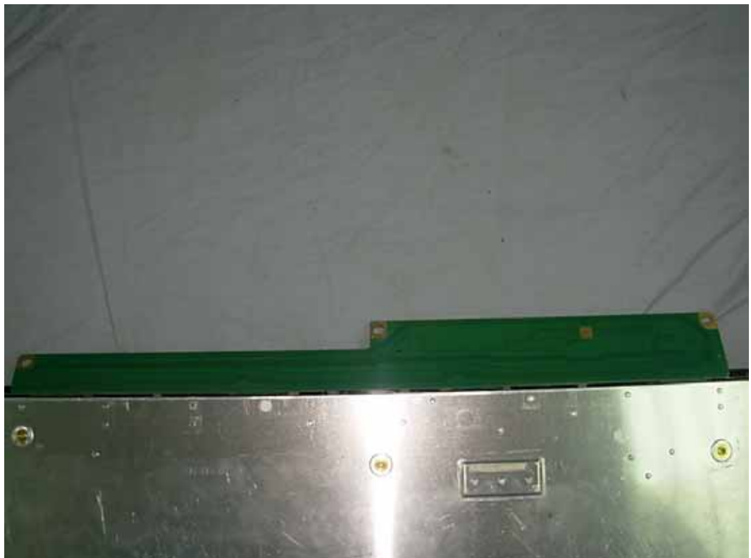
FIGURE 9 LCD MONITOR (M/N: E2210TW) DISPLAY BOARD (SOLDERED SIDE)
