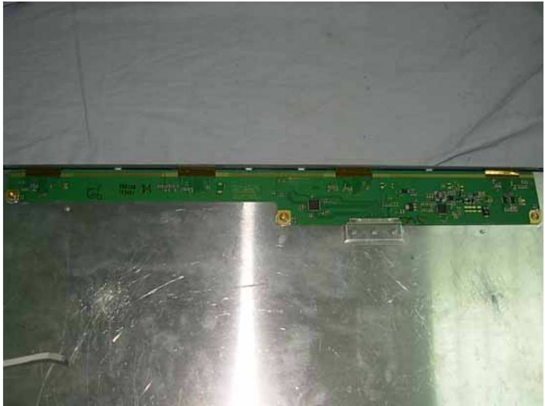
FIGURE 8 LCD MONITOR (M/N: E2210TW) DISPLAY BOARD (COMPONENT SIDE)
