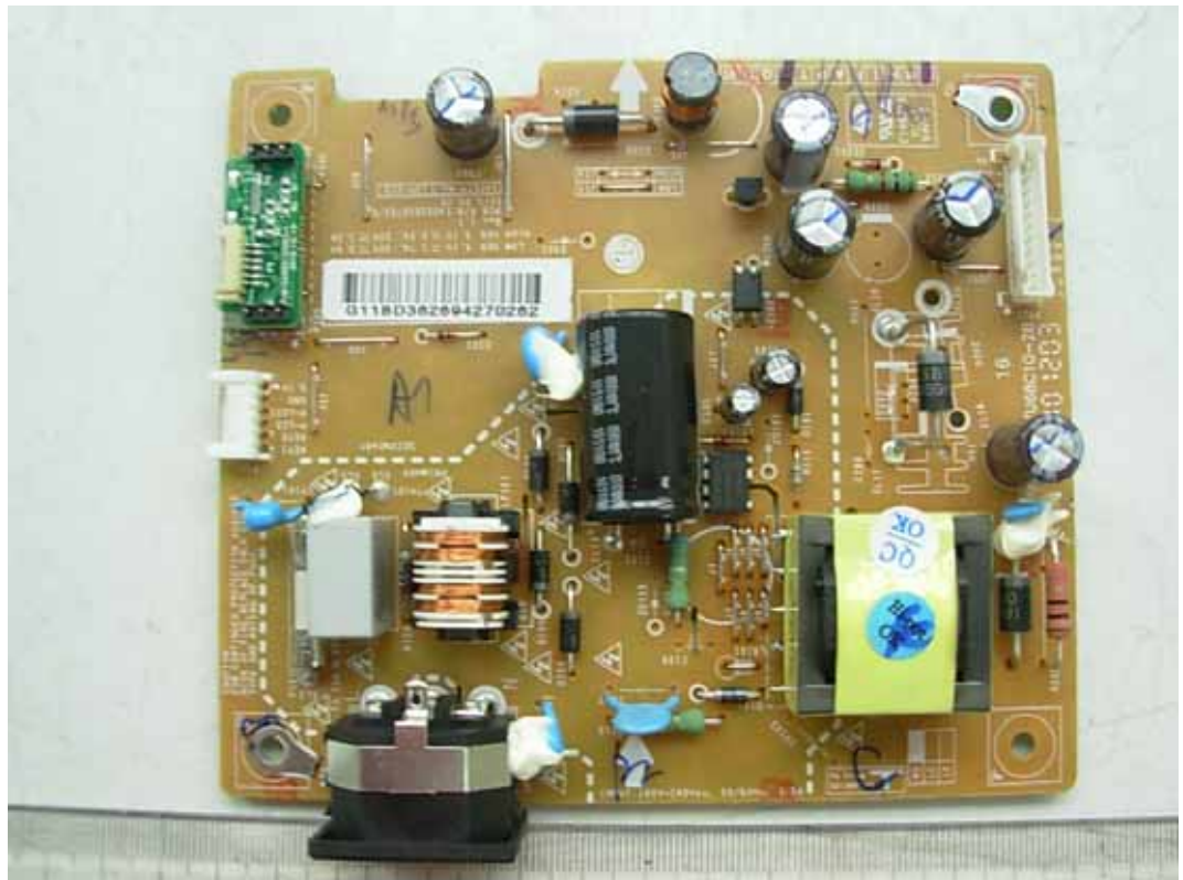
FIGURE 3 LCD MONITOR (M/N: E2211TX) POWER BOARD (COMPONENT SIDE)
