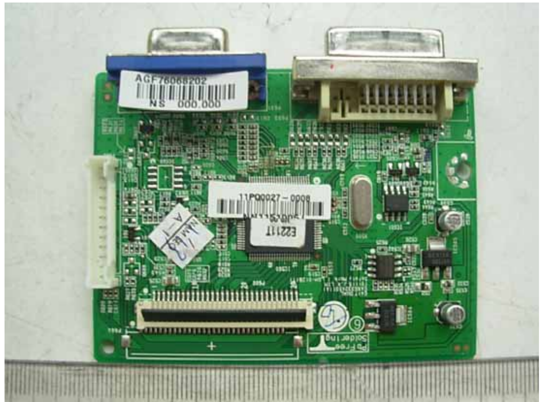
FIGURE 5 LCD MONITOR (M/N: E2211TX) MAIN BOARD (COMPONENT SIDE)
