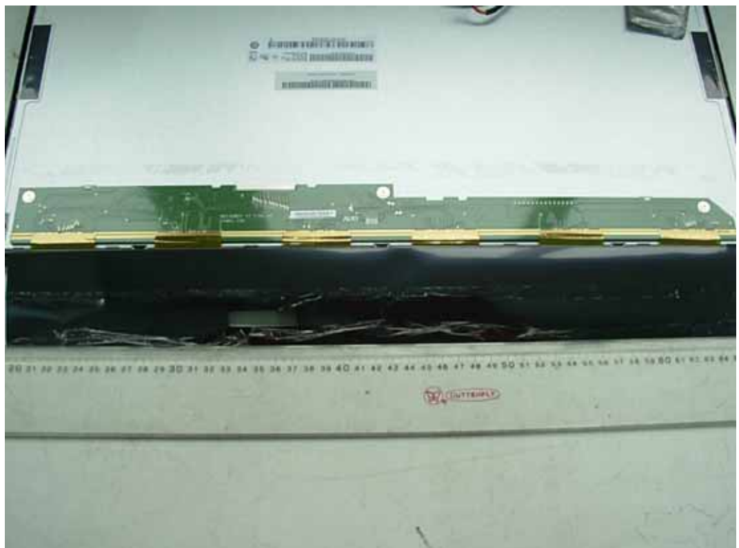
FIGURE 9 LCD MONITOR (M/N: E2211TX) DISPLAY BOARD (SOLDERED SIDE)
