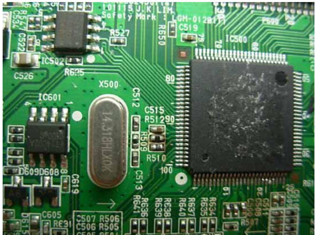
FIGURE 7 LCD MONITOR (M/N: E2211TX) CHIP & CRYSTAL ON MAIN BOARD
