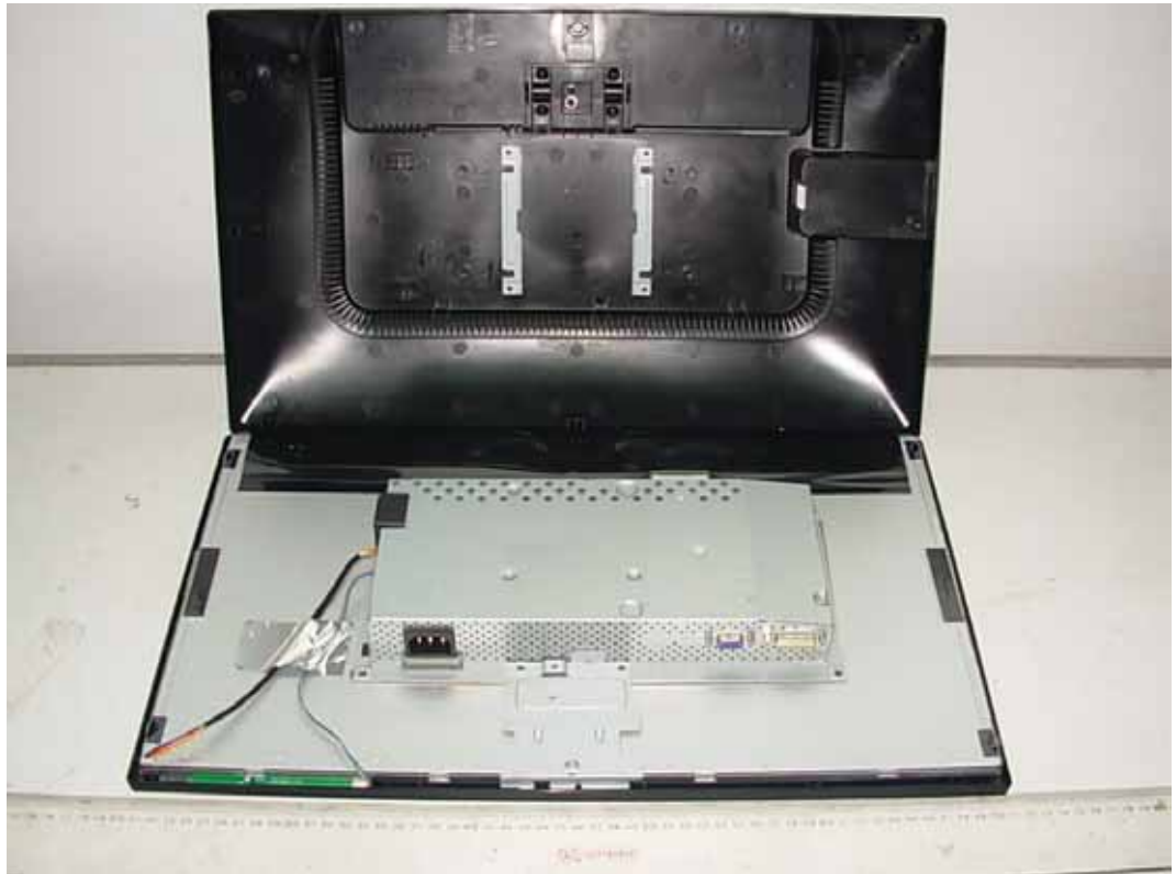
FIGURE 1 LCD MONITOR (M/N: E2211TX) COVER REMOVED
