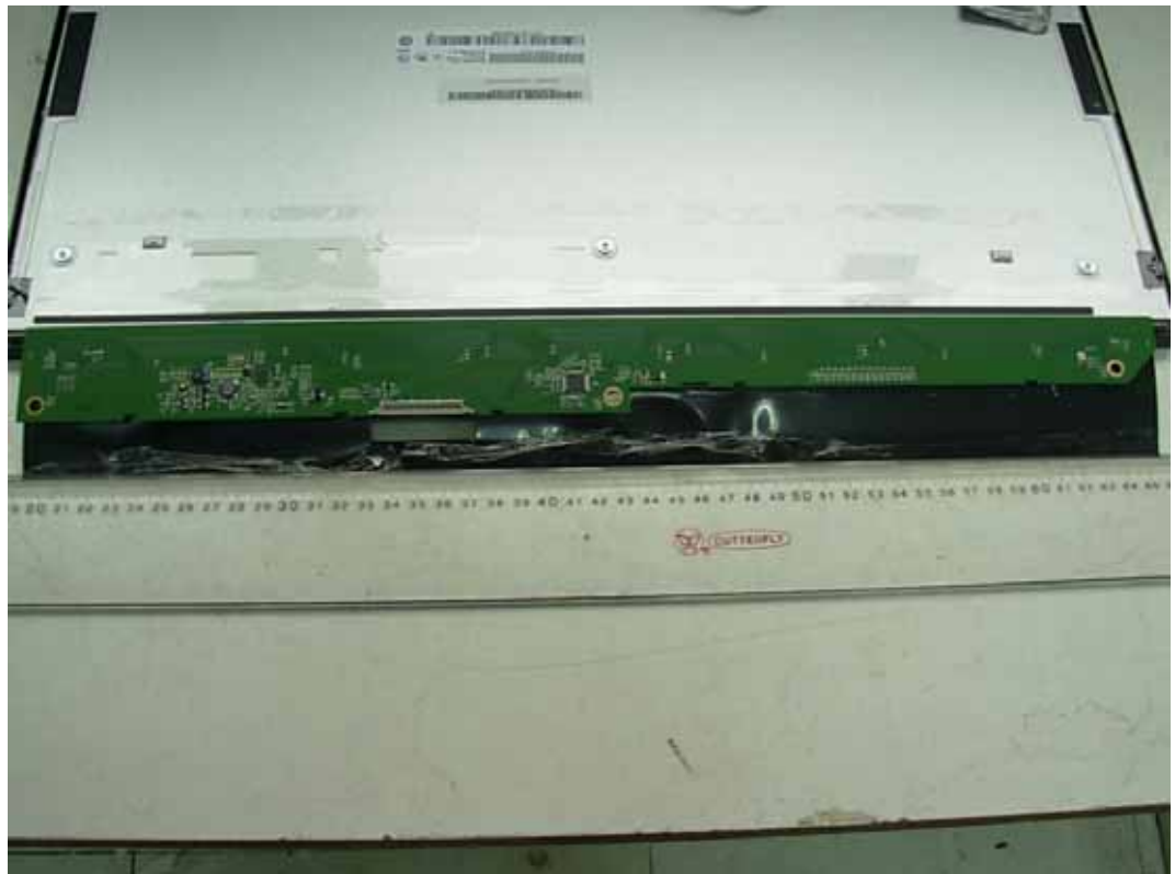
FIGURE 8 LCD MONITOR (M/N: E2211TX) DISPLAY BOARD (COMPONENT SIDE)
