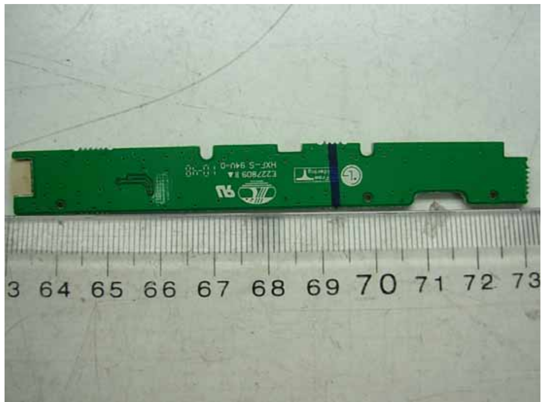
FIGURE 11 LCD MONITOR (M/N: E2211TX) KEY BOARD (SOLDERED SIDE)
