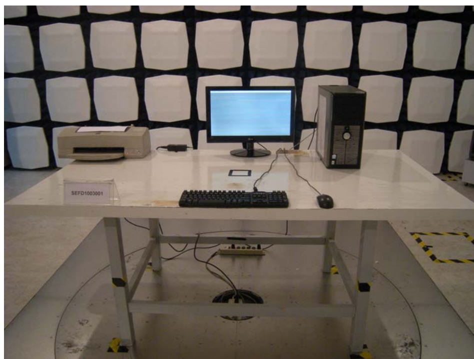
Front View of Radiated Emission Test
