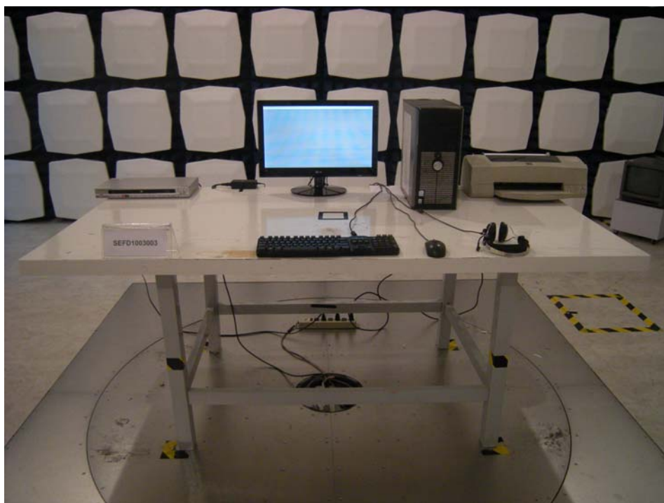
Front View of Radiated Emission Test
