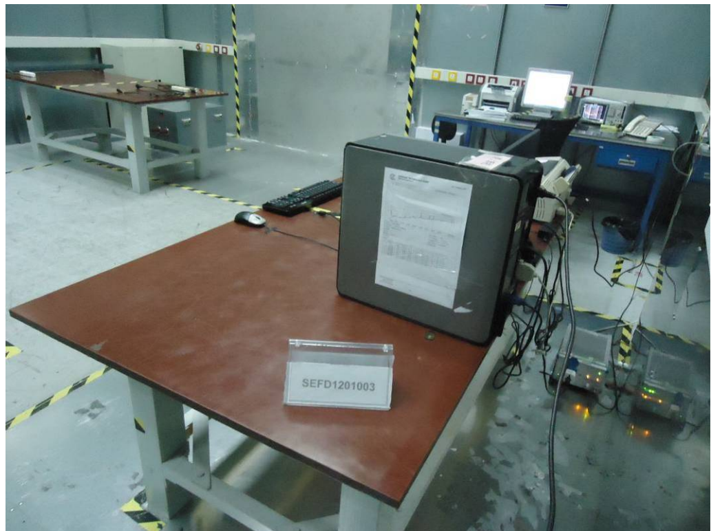
Back View of Conducted Emission Test
