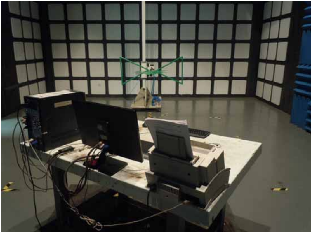
SETUP WITH MAXIMUM DETECTED EMISSION AT HORIZONTAL POLARIZATION (TEST MODE: DVI 1920*1080@60Hz Adapter #1)
