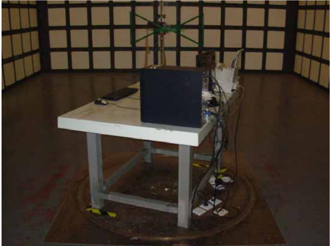
SETUP WITH MAXIMUM DETECTED EMISSION AT HORIZONTAL POLARIZATION (TEST MODE: D-SUB 1680*1050@60Hz)
