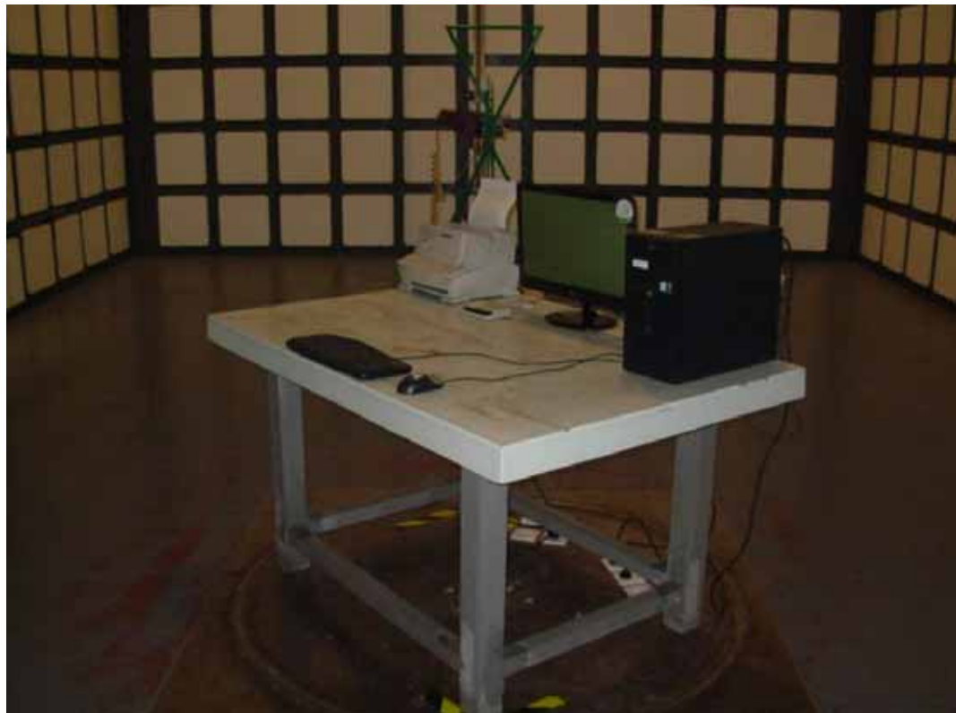
SETUP WITH MAXIMUM DETECTED EMISSION AT VERTICAL POLARIZATION (TEST MODE: D-SUB 1680*1050@60Hz)
