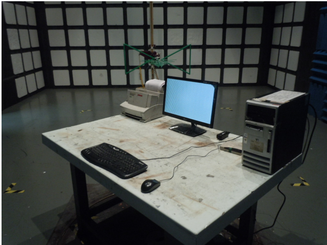
SETUP WITH MAXIMUM DETECTED EMISSION AT HORIZONTAL POLARIZATION (TEST MODE: D-SUB 1920*1080@60Hz Adapter #4)
