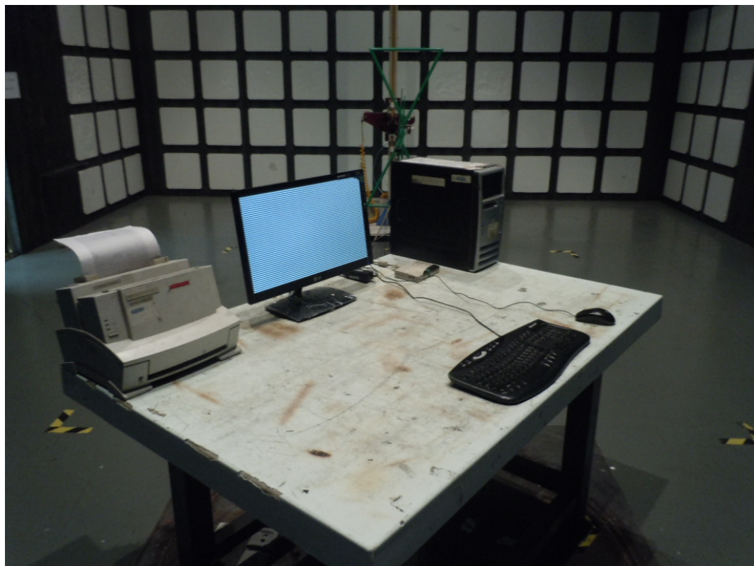
SETUP WITH MAXIMUM DETECTED EMISSION AT VERTICAL POLARIZATION (TEST MODE: D-SUB 1920*1080@60Hz Adapter #4)
