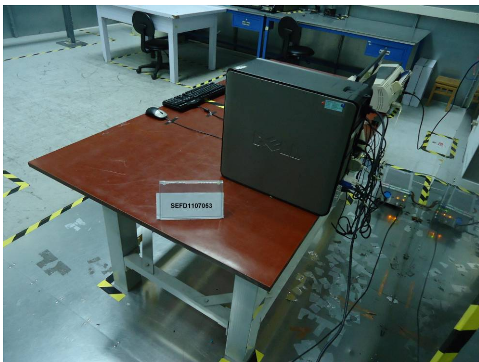
Back View of Conducted Emission Test
