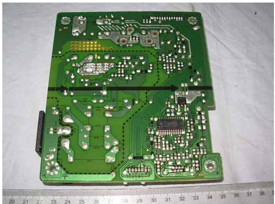
FIGURE 4 LCD MONITOR (M/N: E2341TX) POWER BOARD (SOLDERED SIDE)
