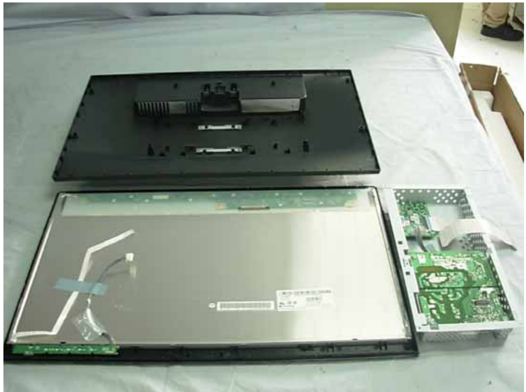
FIGURE 1 LCD MONITOR (M/N: E2341TX) COVER REMOVED
