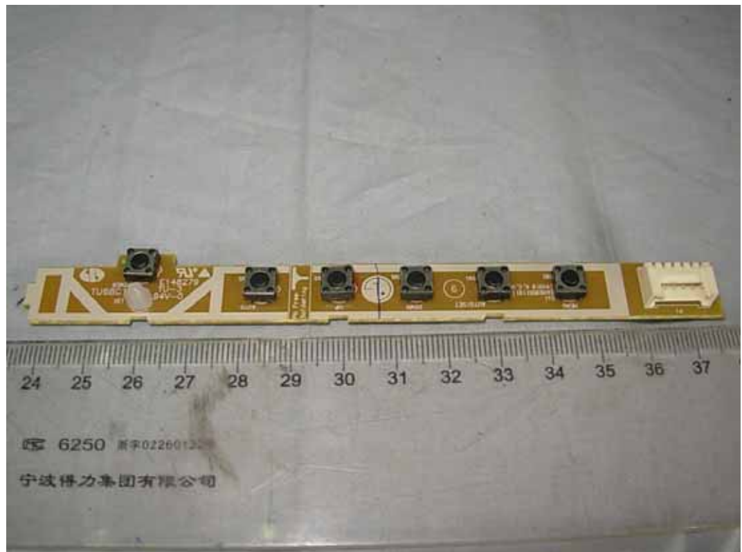
FIGURE 10 LCD MONITOR (M/N: E2341TX) KEY BOARD (COMPONENT SIDE)
