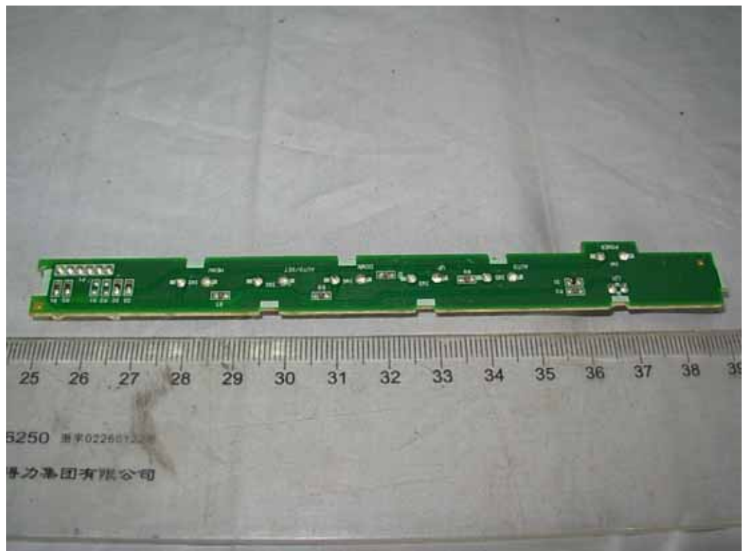
FIGURE 11 LCD MONITOR (M/N: E2341TX) KEY BOARD (SOLDERED SIDE)
