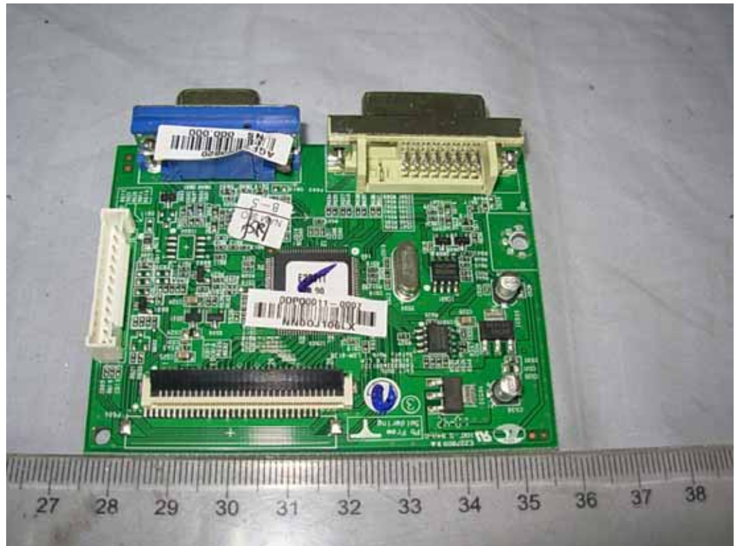
FIGURE 5 LCD MONITOR (M/N: E2341TX) MAIN BOARD (COMPONENT SIDE)
