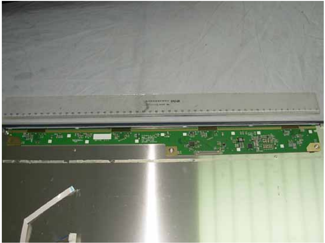
FIGURE 8 LCD MONITOR (M/N: E2341TX) DISPLAY BOARD (COMPONENT SIDE)
