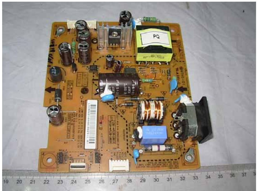
FIGURE 3 LCD MONITOR (M/N: E2341TX) POWER BOARD (COMPONENT SIDE)
