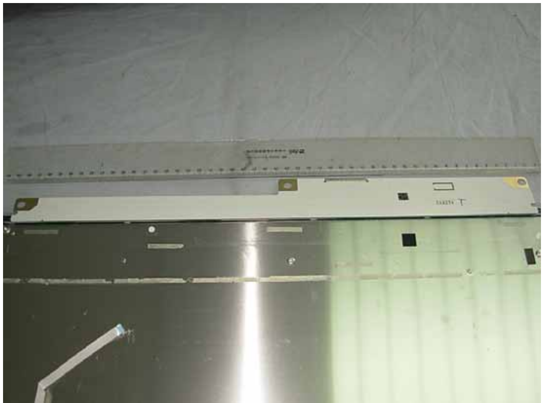
FIGURE 9 LCD MONITOR (M/N: E2341TX) DISPLAY BOARD (SOLDERED SIDE)
