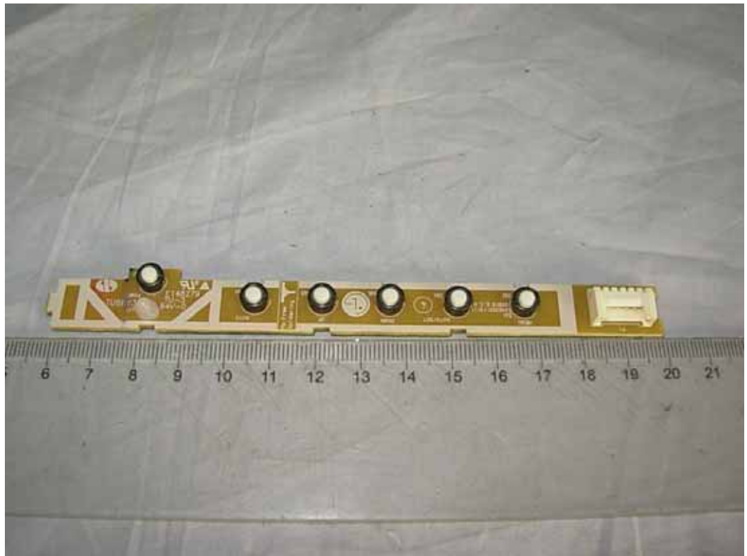
FIGURE 10 LCD MONITOR (M/N: E2341VX) KEY BOARD (COMPONENT SIDE)
