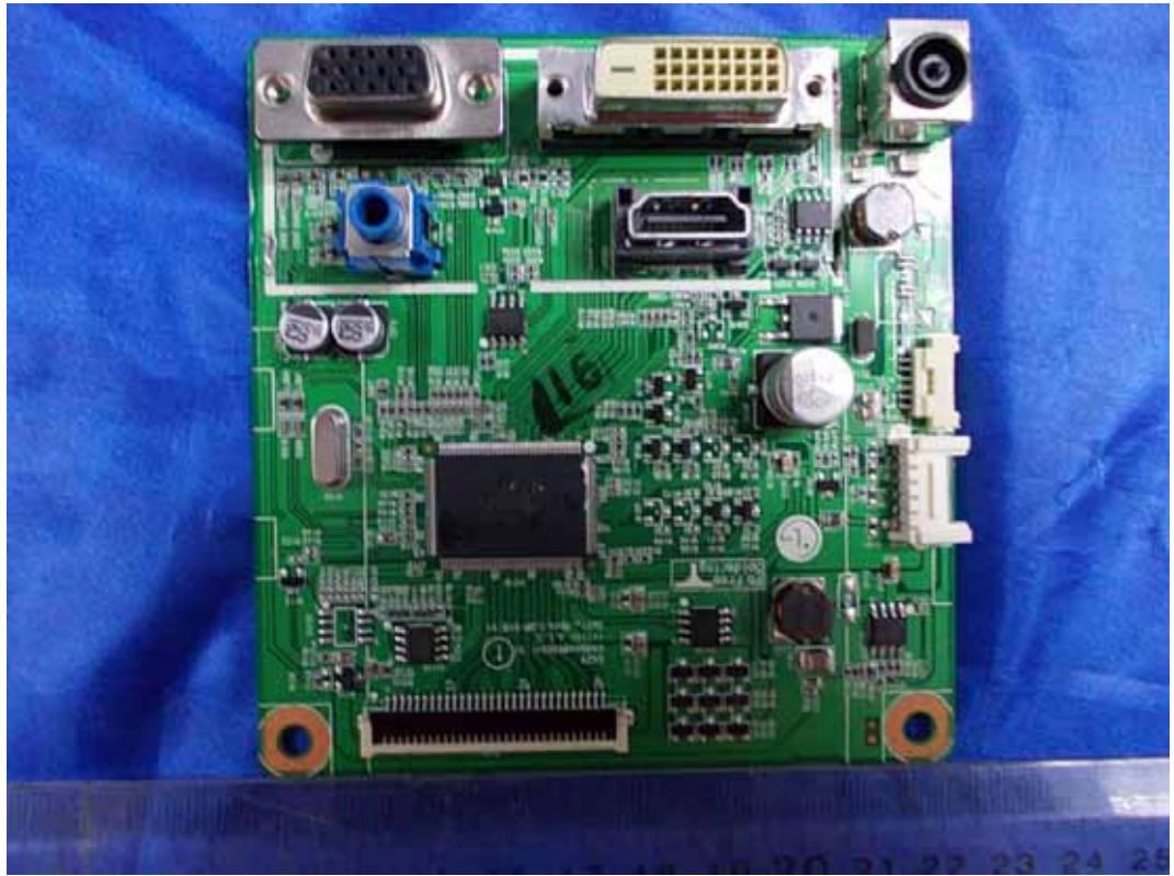
FIGURE 3 LCD MONITOR (M/N: E2342VA) MAIN BOARD (COMPONENT SIDE)
