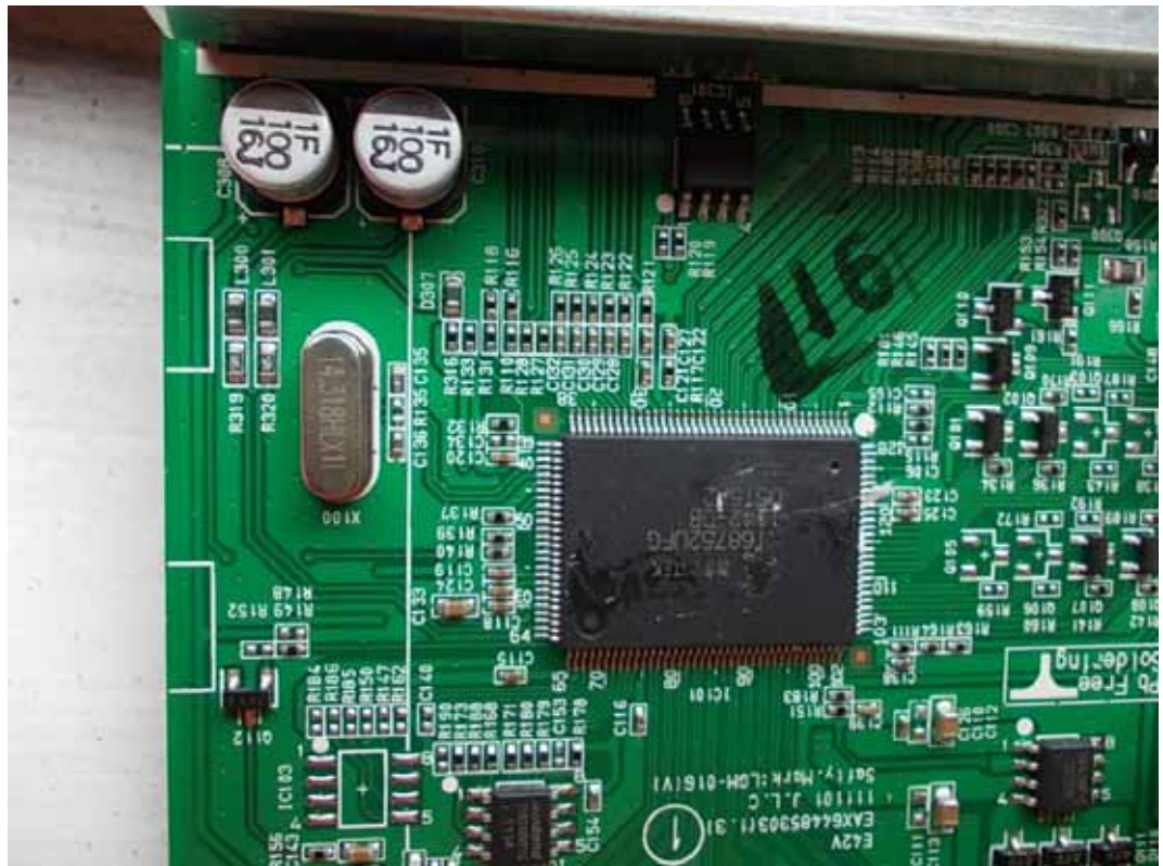
FIGURE 5 LCD MONITOR (M/N: E2342VA) CHIP & CRYSTAL ON MAIN BOARD
