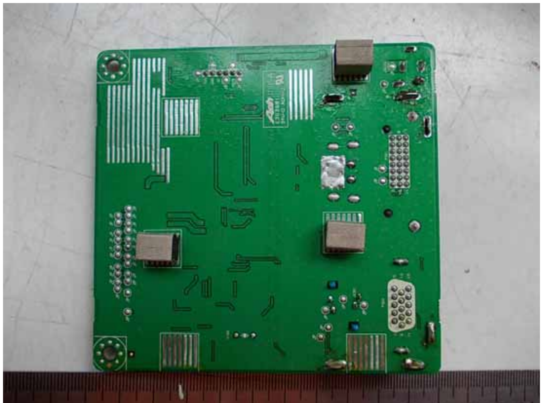
FIGURE 4 LCD MONITOR (M/N: E2342VA) MAIN BOARD (COMPONENT SIDE)
