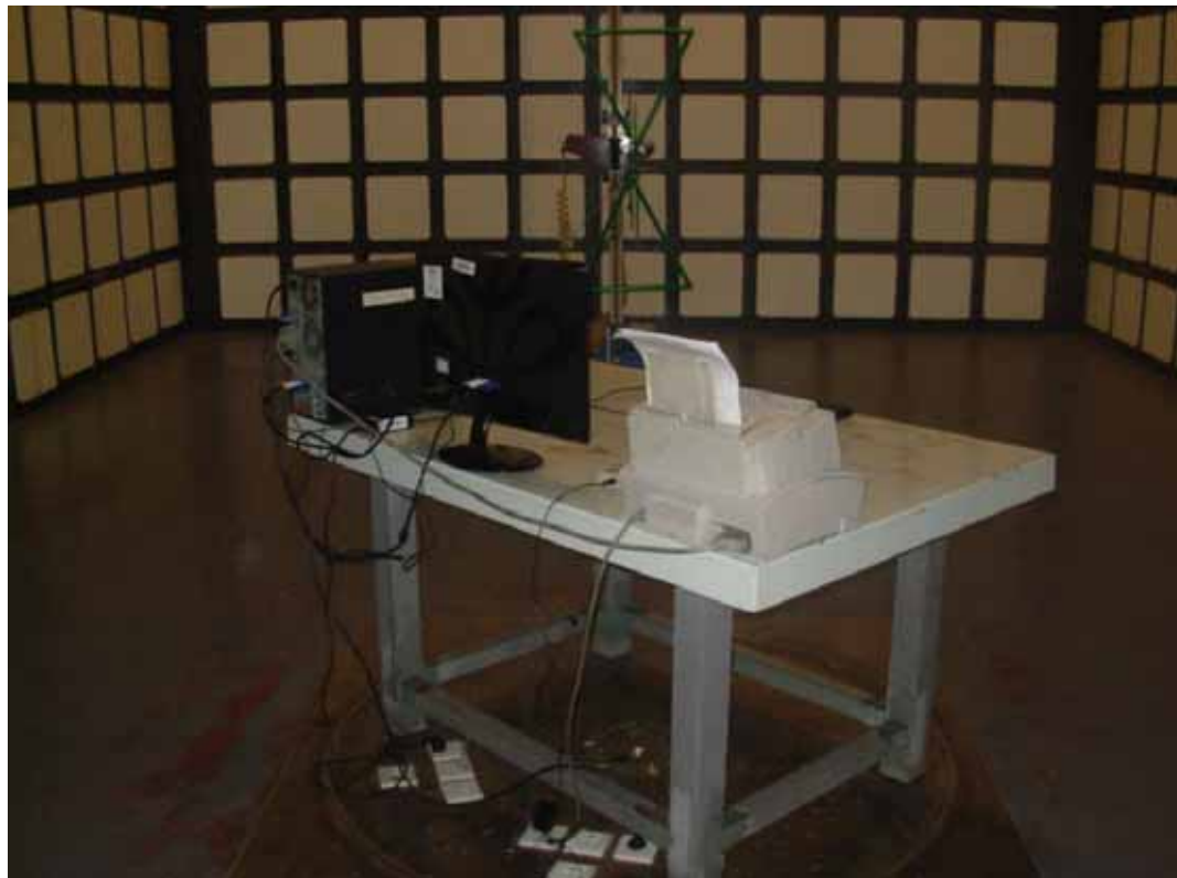
SETUP WITH MAXIMUM DETECTED EMISSION AT VERTICAL POLARIZATION (TEST MODE: DVI 1280*1024@75Hz) (ADAPTER: FSP036-DGAA1)
