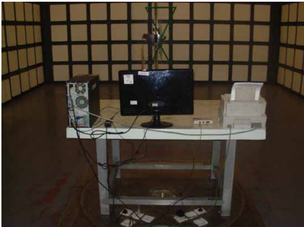
BACK VIEW OF RADIATED EMISSION TEST
