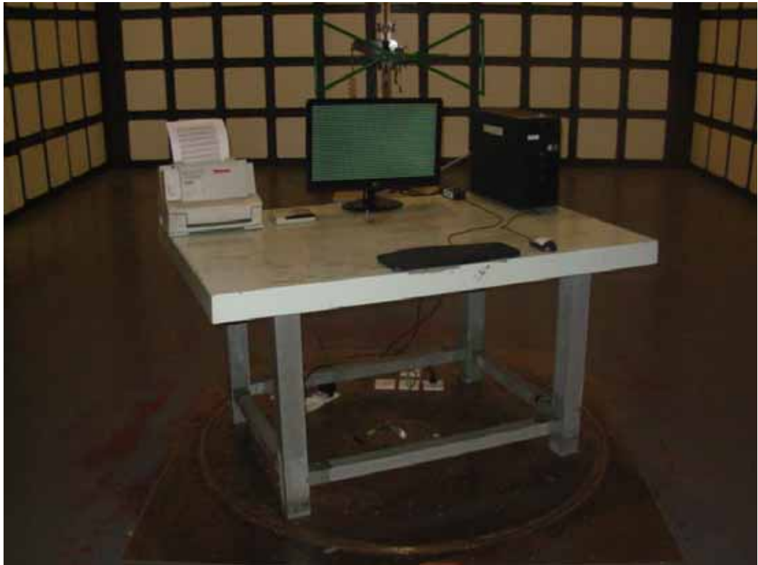
SETUP WITH MAXIMUM DETECTED EMISSION AT HORIZONTAL POLARIZATION (TEST MODE: DVI 1280*1024@75Hz) (ADAPTER: FSP036-DGAA1)
