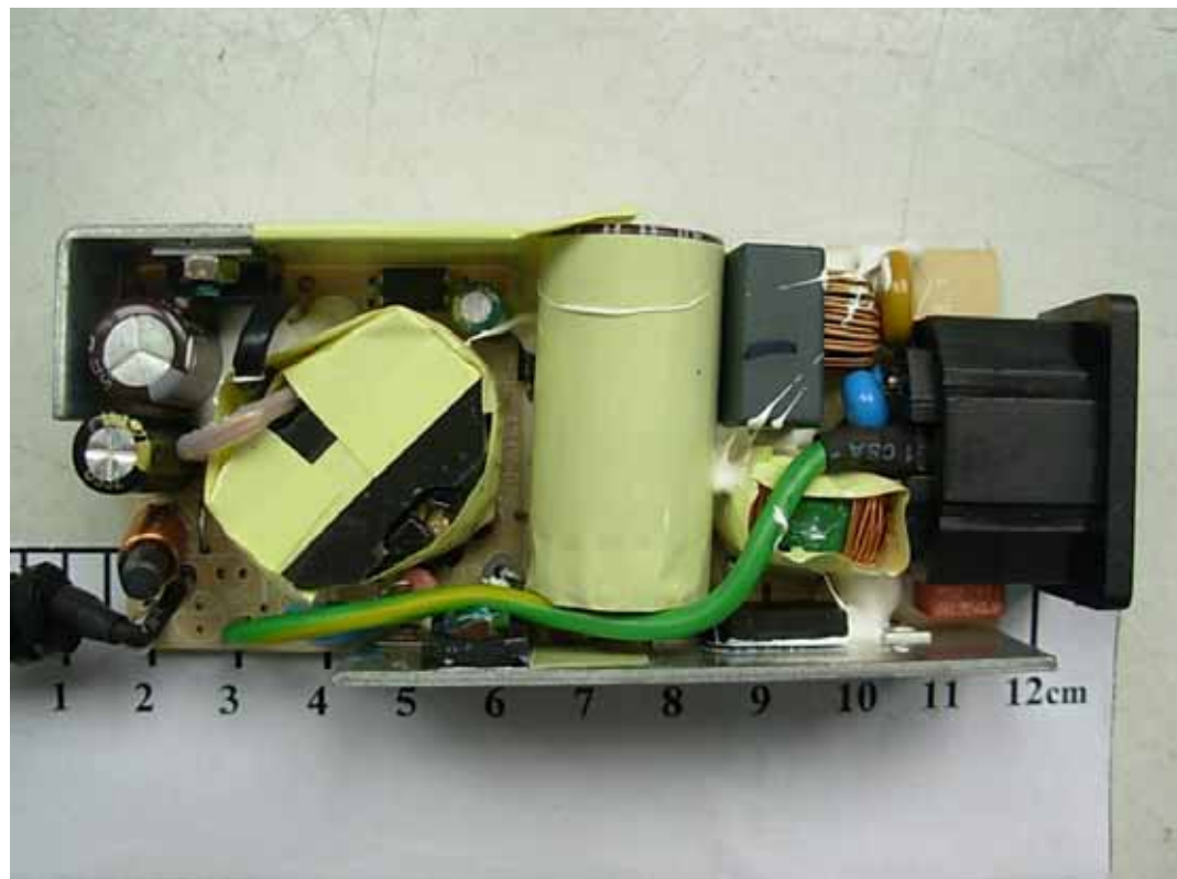
FIGURE 20 LCD MONITOR (M/N: E2350VV) ADAPTER #2 (MAIN BOARD – COMPONENT SIDE)
