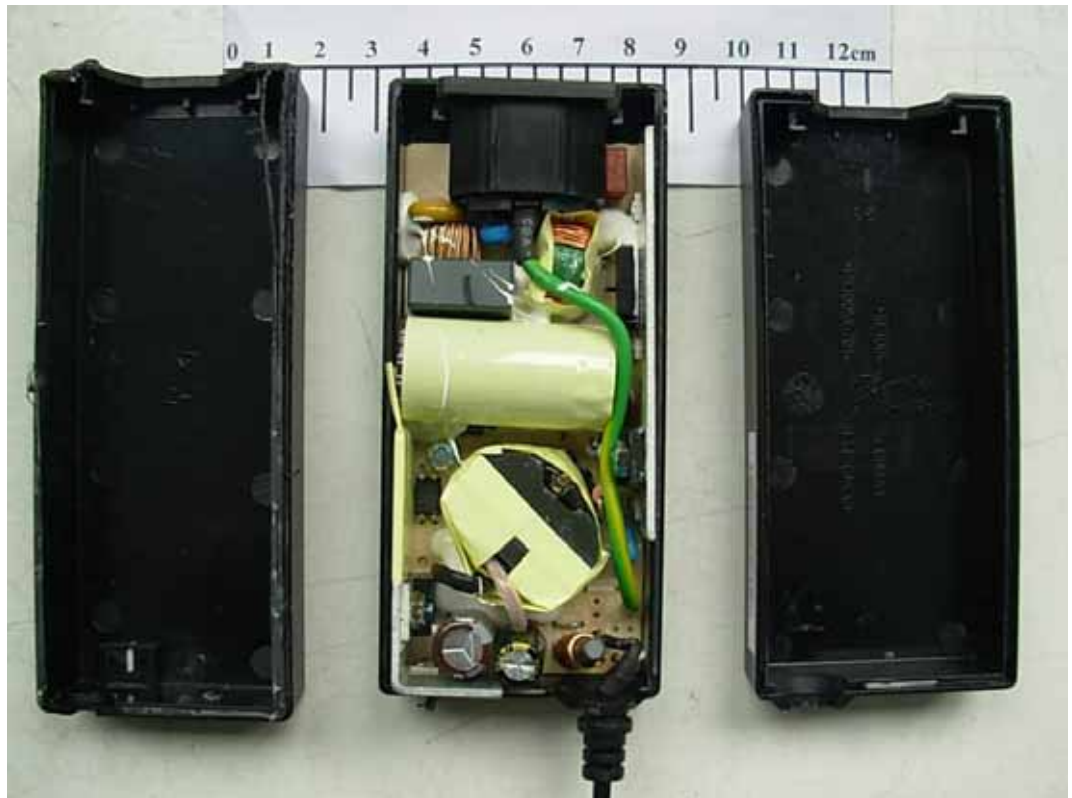
FIGURE 19 LCD MONITOR (M/N: E2350VV) ADAPTER #2 (COVER REMOVED)
