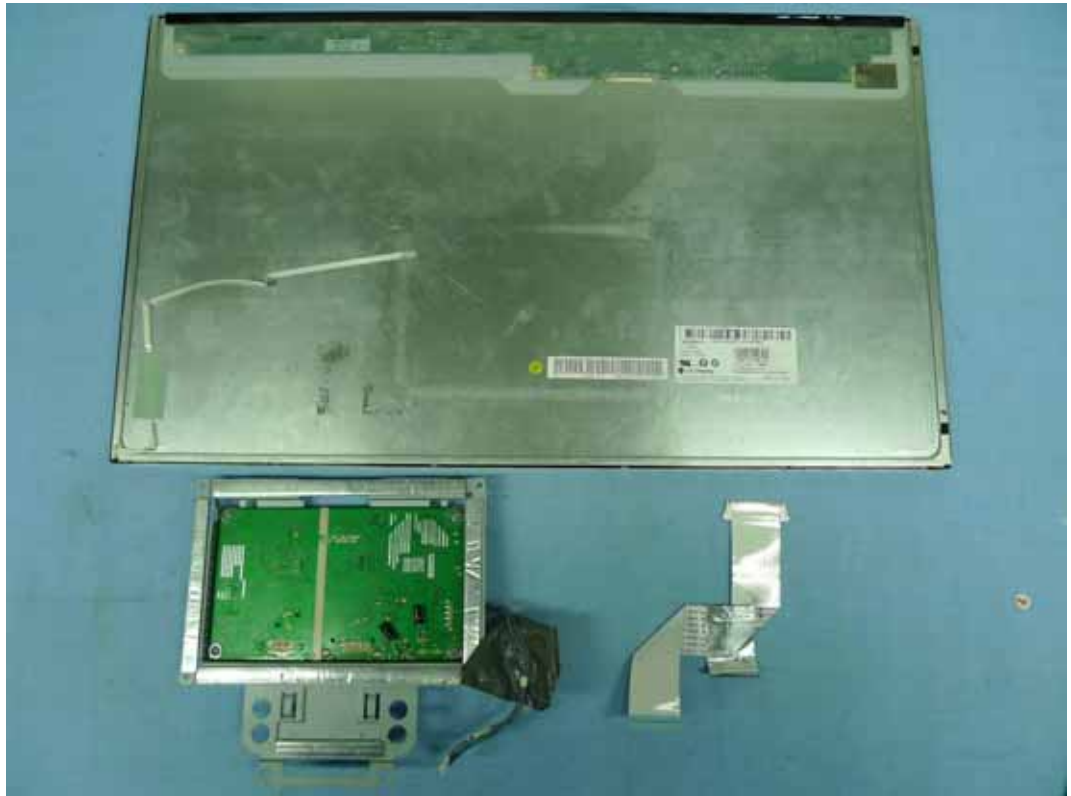
FIGURE 4 LCD MONITOR (M/N: E2350VV) BOARDS REMOVED
