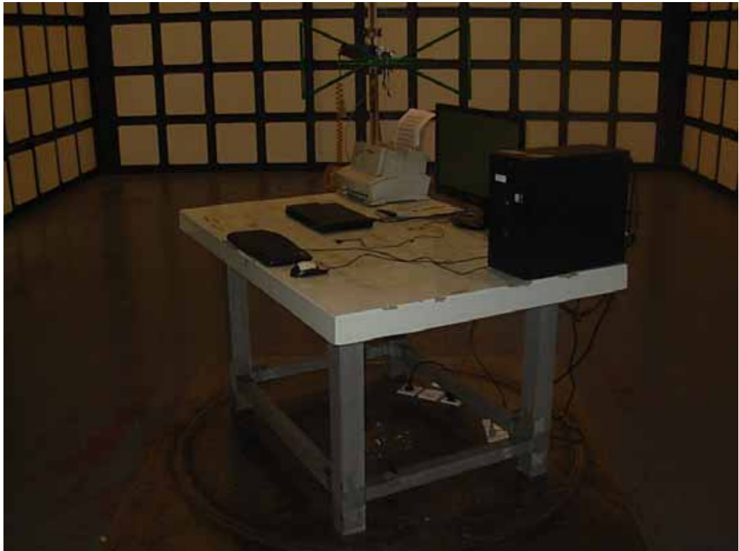
SETUP WITH MAXIMUM DETECTED EMISSION AT HORIZONTAL POLARIZATION (TEST MODE: D-SUB 1680*1050@60Hz) (ADAPTER: LCAP07F)
