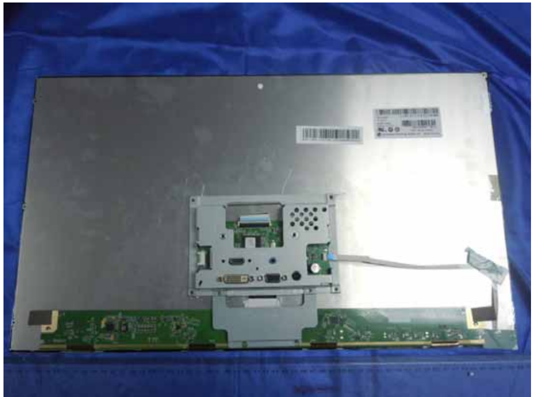
FIGURE 1 LCD MONITOR (M/N: E2351VZ) COVER REMOVED
