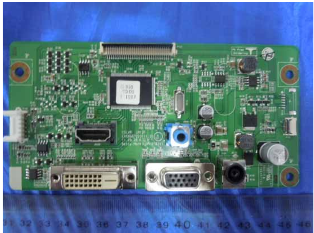
FIGURE 3 LCD MONITOR (M/N: E2351VZ) MAIN BOARD (COMPONENT SIDE)
