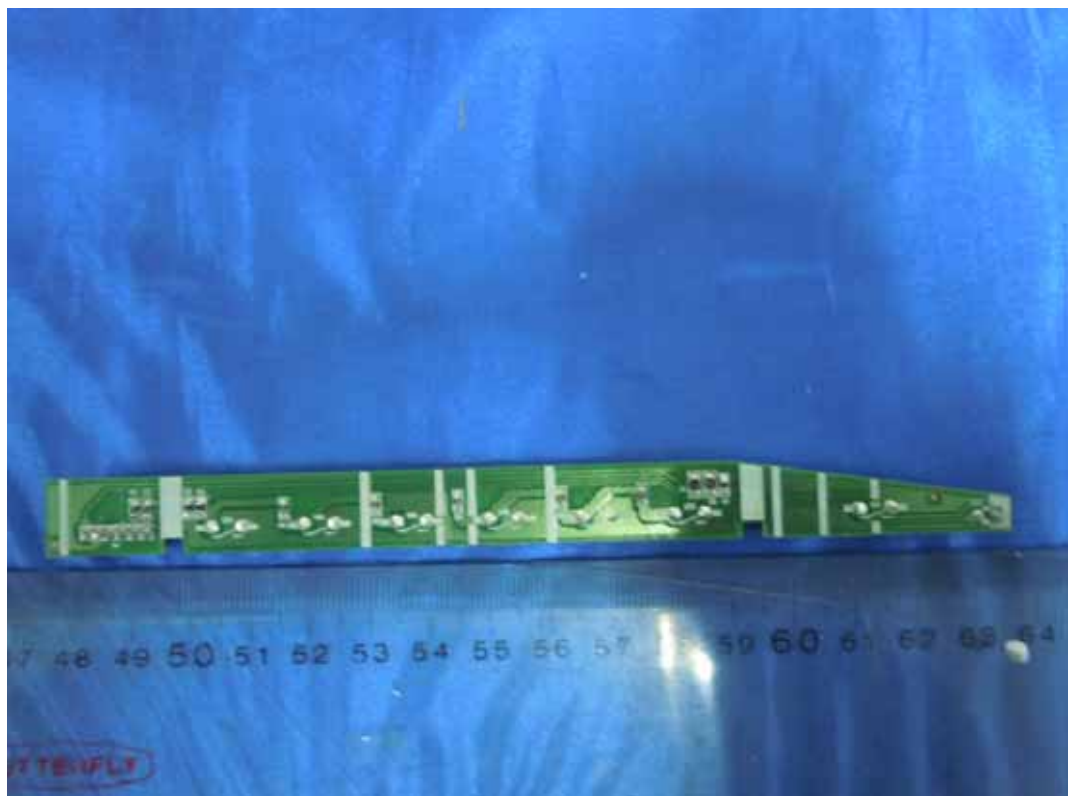
FIGURE 7 LCD MONITOR (M/N: E2351VZ) KEY BOARD (SOLDERED SIDE)
