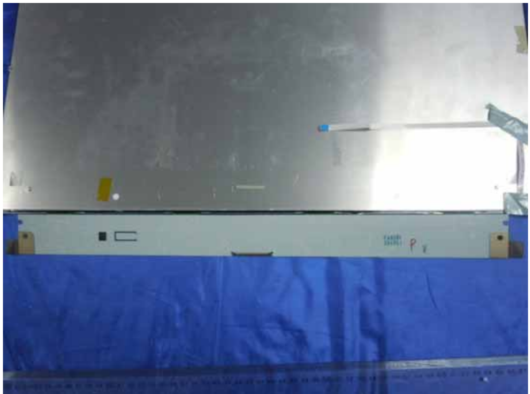
FIGURE 9 LCD MONITOR (M/N: E2351VZ) LCD PANEL CONTROL BOARD (SOLDERED SIDE)
