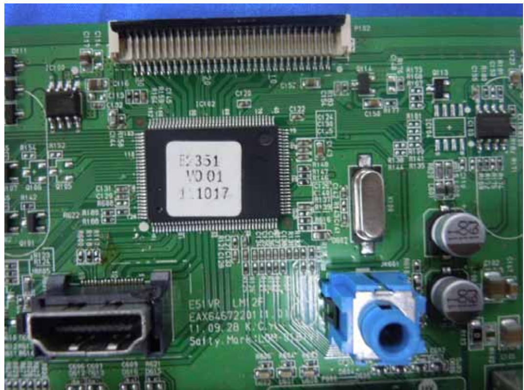
FIGURE 5 LCD MONITOR (M/N: E2351VZ) CHIP & CRYSTAL ON MAIN BOARD
