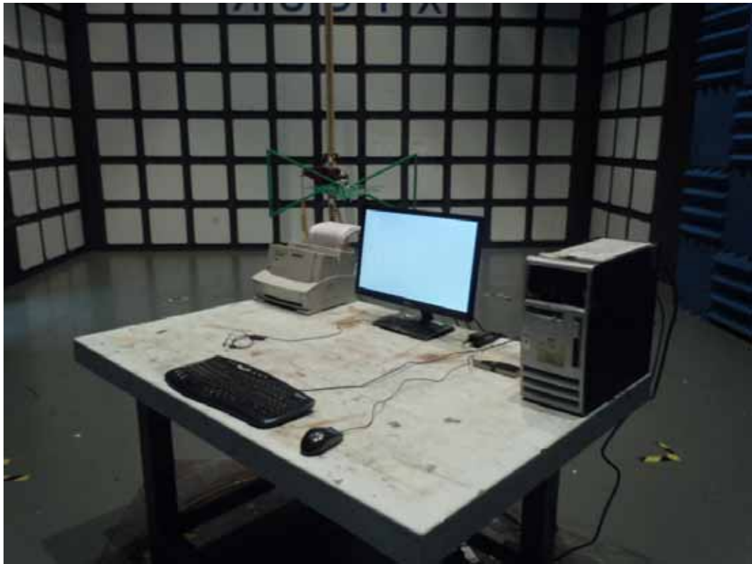
SETUP WITH MAXIMUM DETECTED EMISSION AT HORIZONTAL POLARIZATION (TEST MODE: D-SUB 1920*1080@60Hz Adapter #1)
