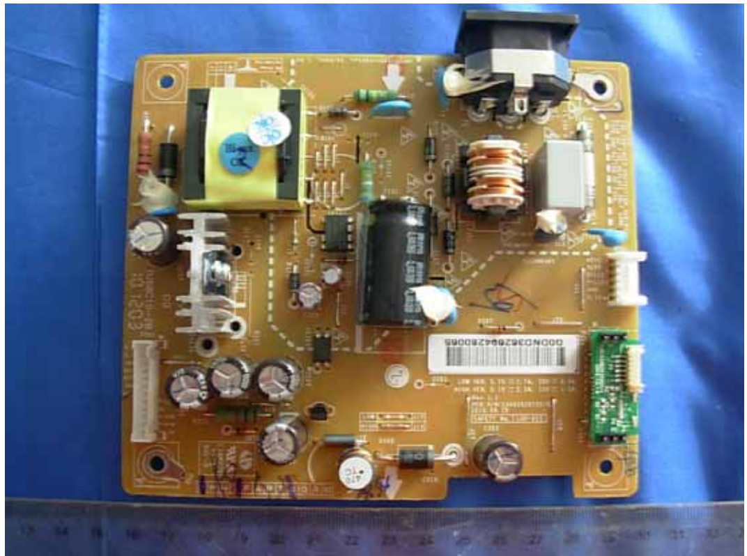
FIGURE 6 LCD MONITOR (M/N: E2411PUX) POWER BOARD (COMPONENT SIDE)
