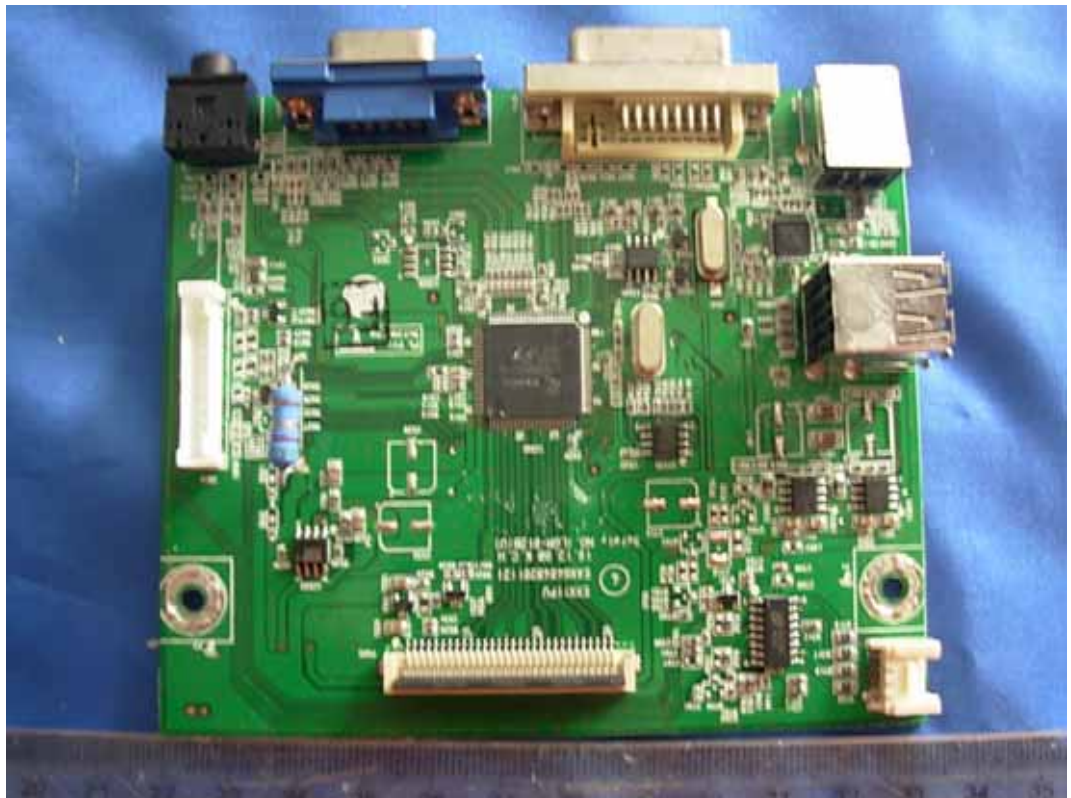
FIGURE 3 LCD MONITOR (M/N: E2411PUX) MAIN BOARD (COMPONENT SIDE)
