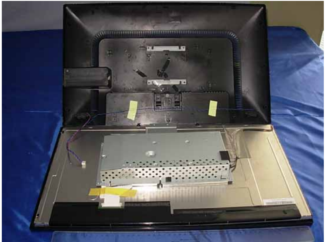
FIGURE 1 LCD MONITOR (M/N: E2411PUX) COVER REMOVED
