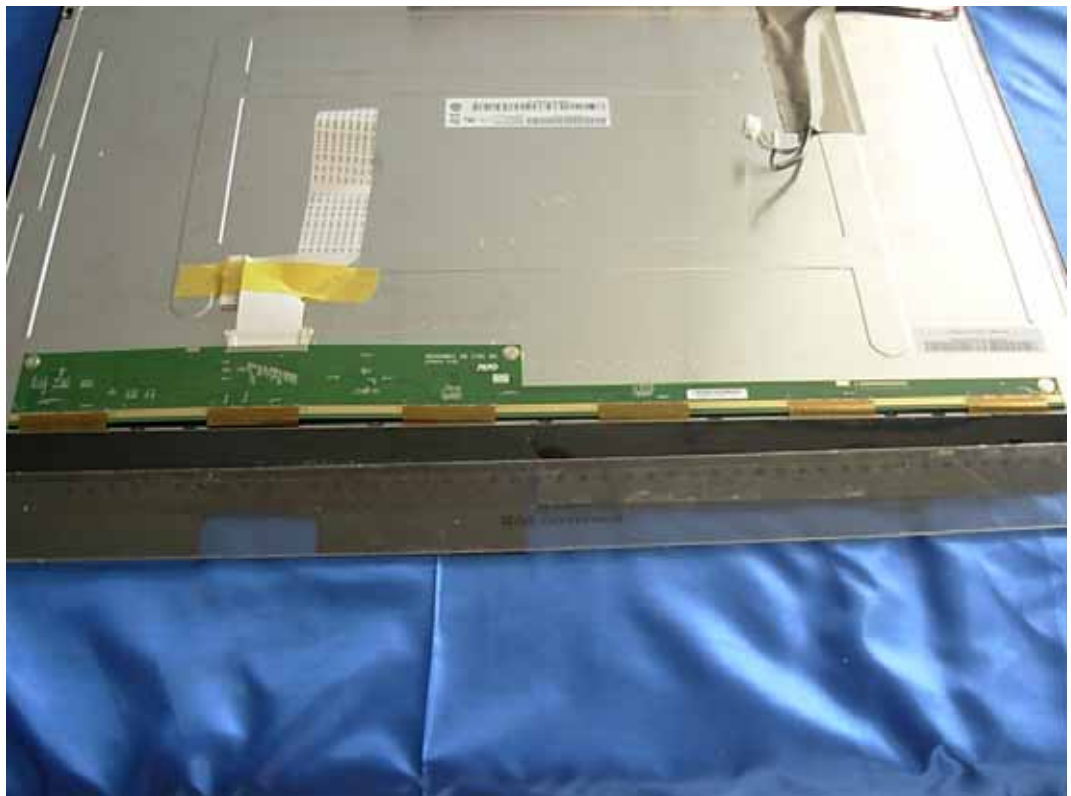
FIGURE 9 LCD MONITOR (M/N: E2411PUX) LCD PANEL BOARD (SOLDERED SIDE)
