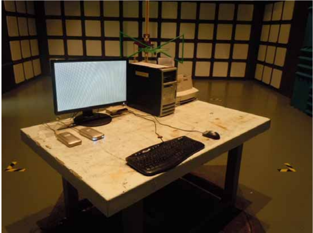
SETUP WITH MAXIMUM DETECTED EMISSION AT HORIZONTAL POLARIZATION (TEST MODE: DVI 1680*1050@60Hz)
