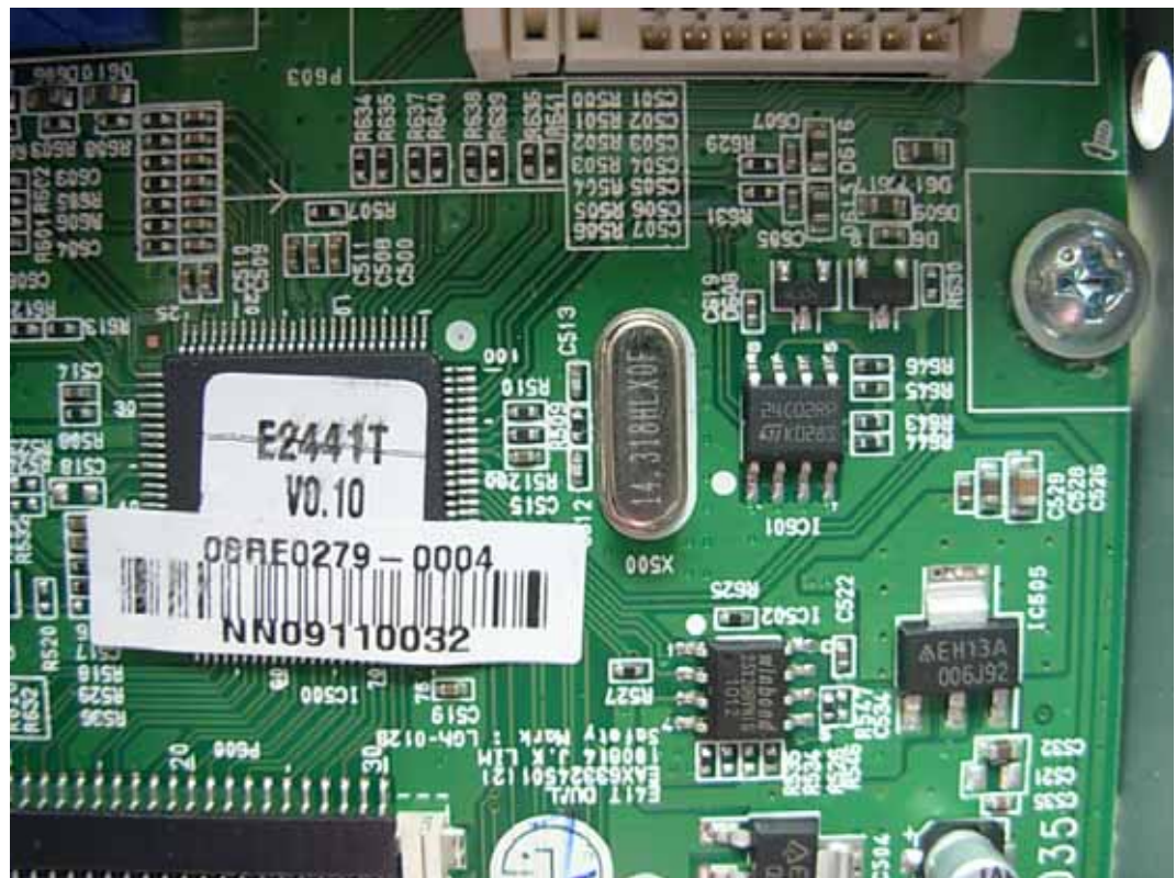
FIGURE 7 LCD MONITOR (M/N: E2441TX) CHIP & CRYSTAL ON MAIN BOARD
