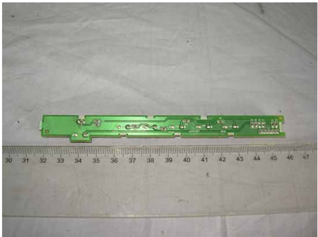
FIGURE 11 LCD MONITOR (M/N: E2441TX) KEY BOARD (SOLDERED SIDE)
