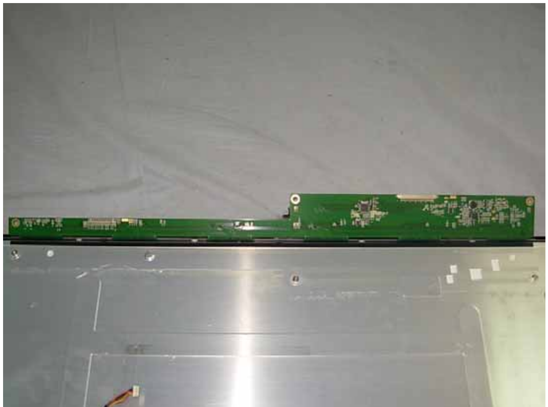
FIGURE 9 LCD MONITOR (M/N: E2441TX) DISPLAY BOARD (SOLDERED SIDE)
