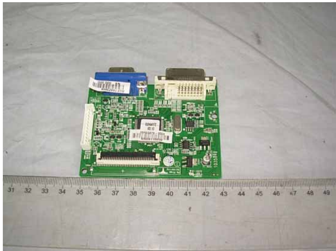
FIGURE 5 LCD MONITOR (M/N: E2441TX) MAIN BOARD (COMPONENT SIDE)
