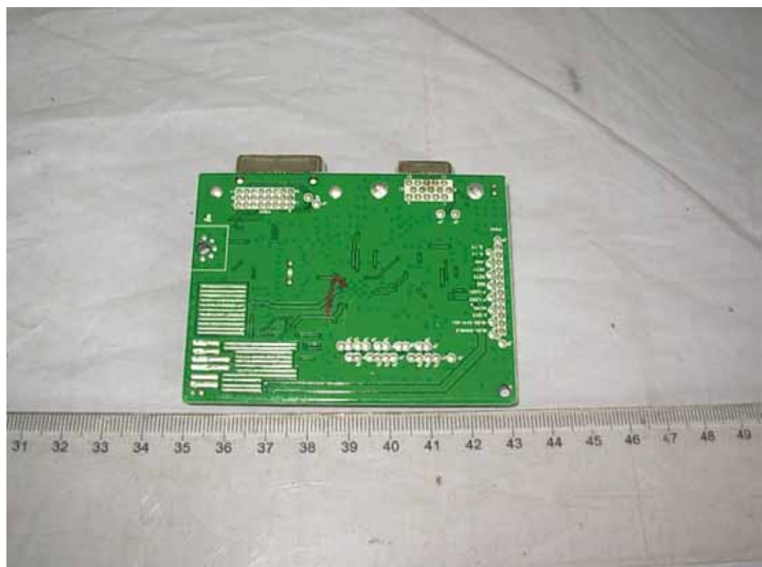
FIGURE 6 LCD MONITOR (M/N: E2441TX) MAIN BOARD (SOLDERED SIDE)
