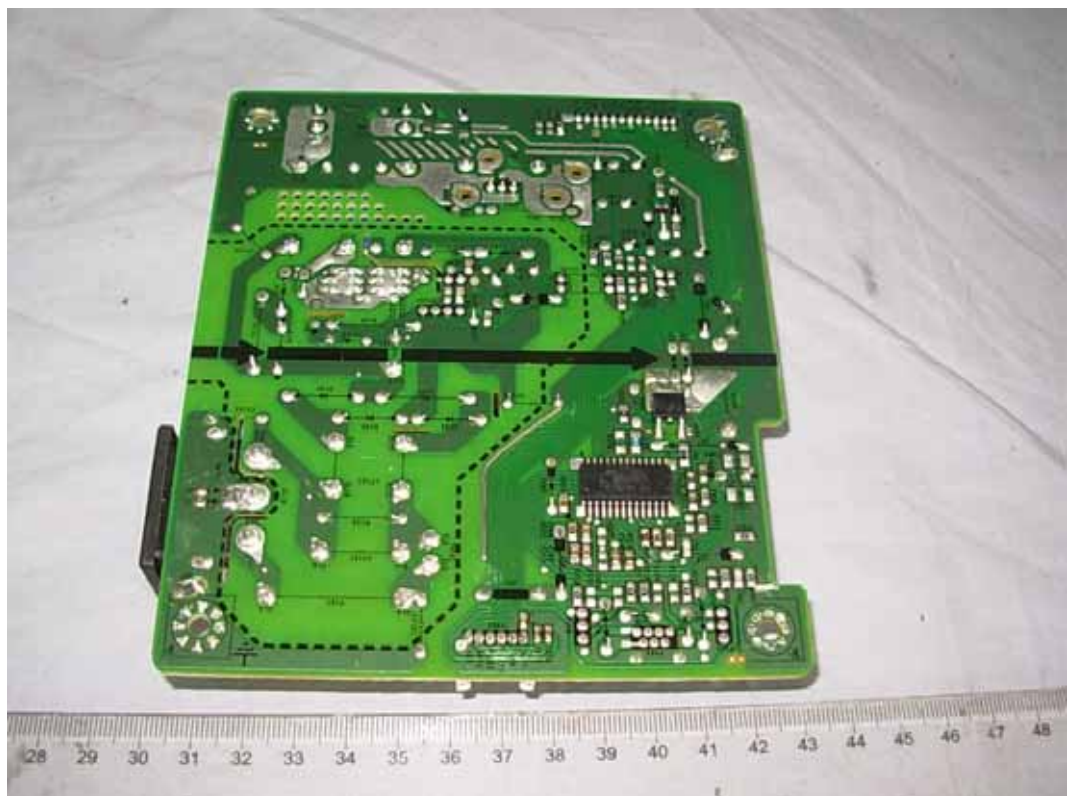
FIGURE 4 LCD MONITOR (M/N: E2441TX) POWER BOARD (COMPONENT SIDE)
