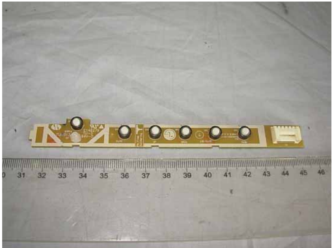
FIGURE 10 LCD MONITOR (M/N: E2441TX) KEY BOARD (COMPONENT SIDE)
