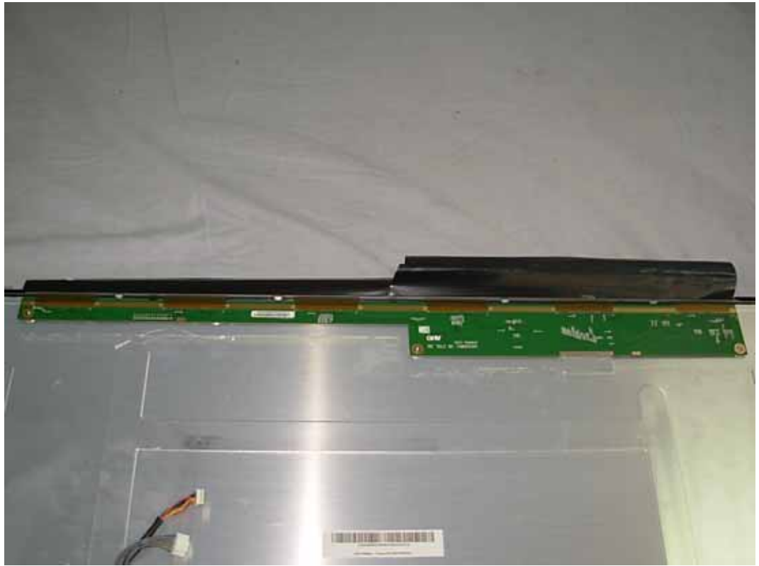
FIGURE 8 LCD MONITOR (M/N: E2441TX) DISPLAY BOARD (COMPONENT SIDE)
