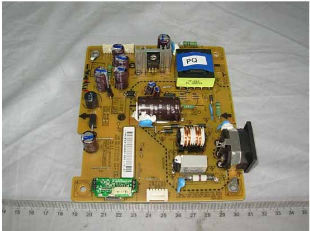
FIGURE 3 LCD MONITOR (M/N: E2441TX) POWER BOARD (COMPONENT SIDE)
