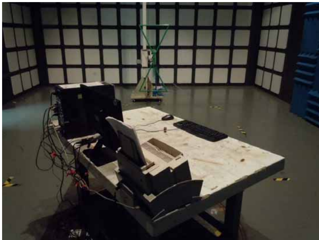
SETUP WITH MAXIMUM DETECTED EMISSION AT VERTICAL POLARIZATION (TEST MODE: DVI 1920*1080@60Hz Adapter #4, Panel #2)
