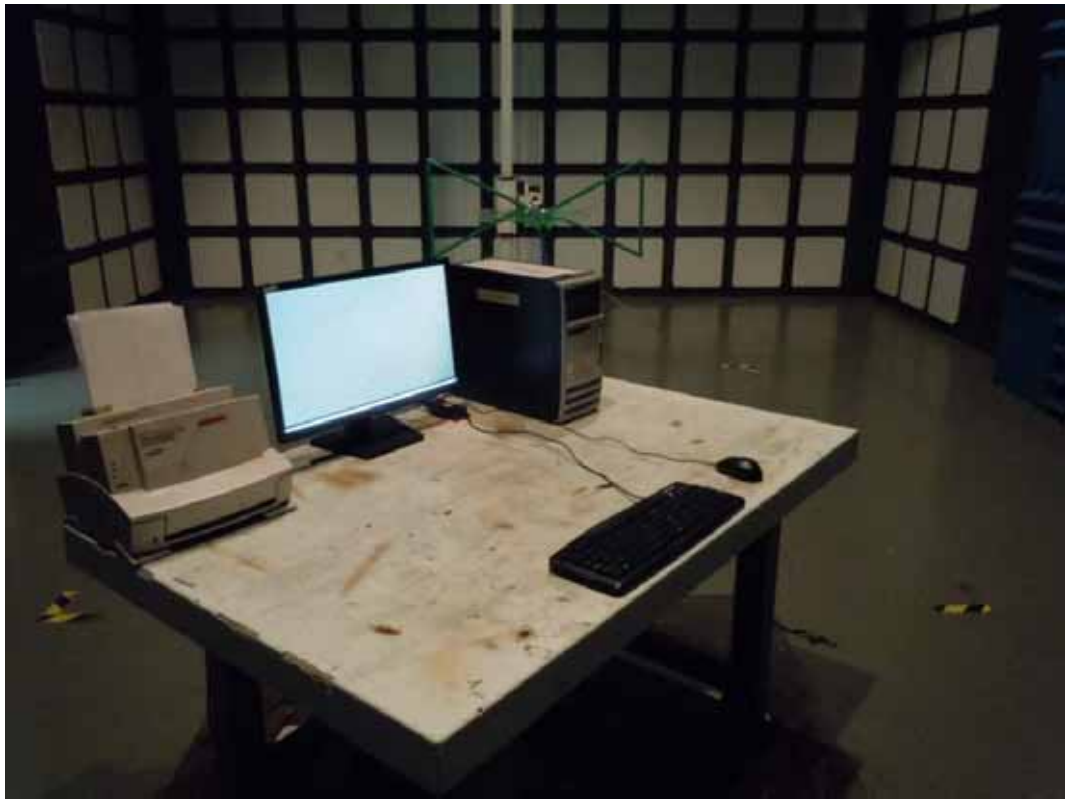
SETUP WITH MAXIMUM DETECTED EMISSION AT HORIZONTAL POLARIZATION (TEST MODE: DVI 1920*1080@60Hz Adapter #4, Panel #2)
