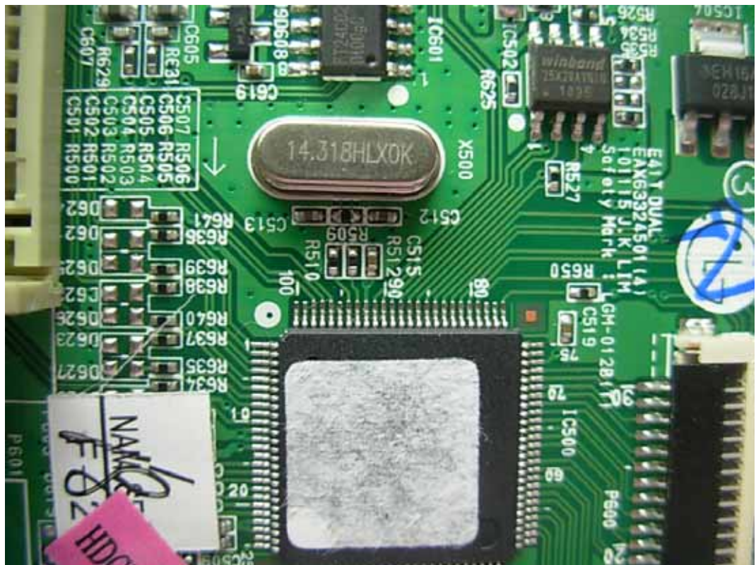
FIGURE 5 LCD MONITOR (M/N: E2541TX) CHIP & CRYSTAL ON MAIN BOARD
