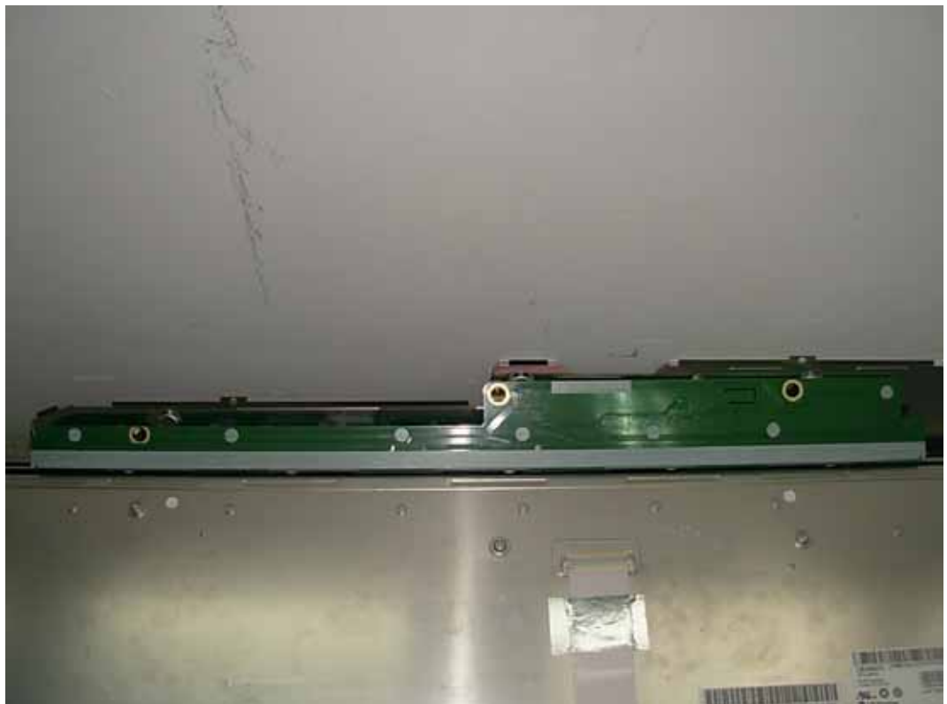
FIGURE 9 LCD MONITOR (M/N: E2541TX) LCD PANEL BOARD (SOLDERED SIDE)
