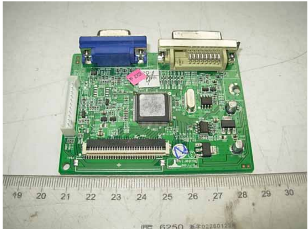
FIGURE 3 LCD MONITOR (M/N: E2541TX) MAIN BOARD (COMPONENT SIDE)
