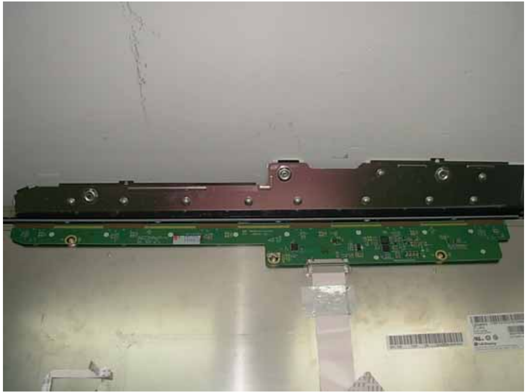
FIGURE 8 LCD MONITOR (M/N: E2541TX) DISPLAY BOARD (COMPONENT SIDE)
