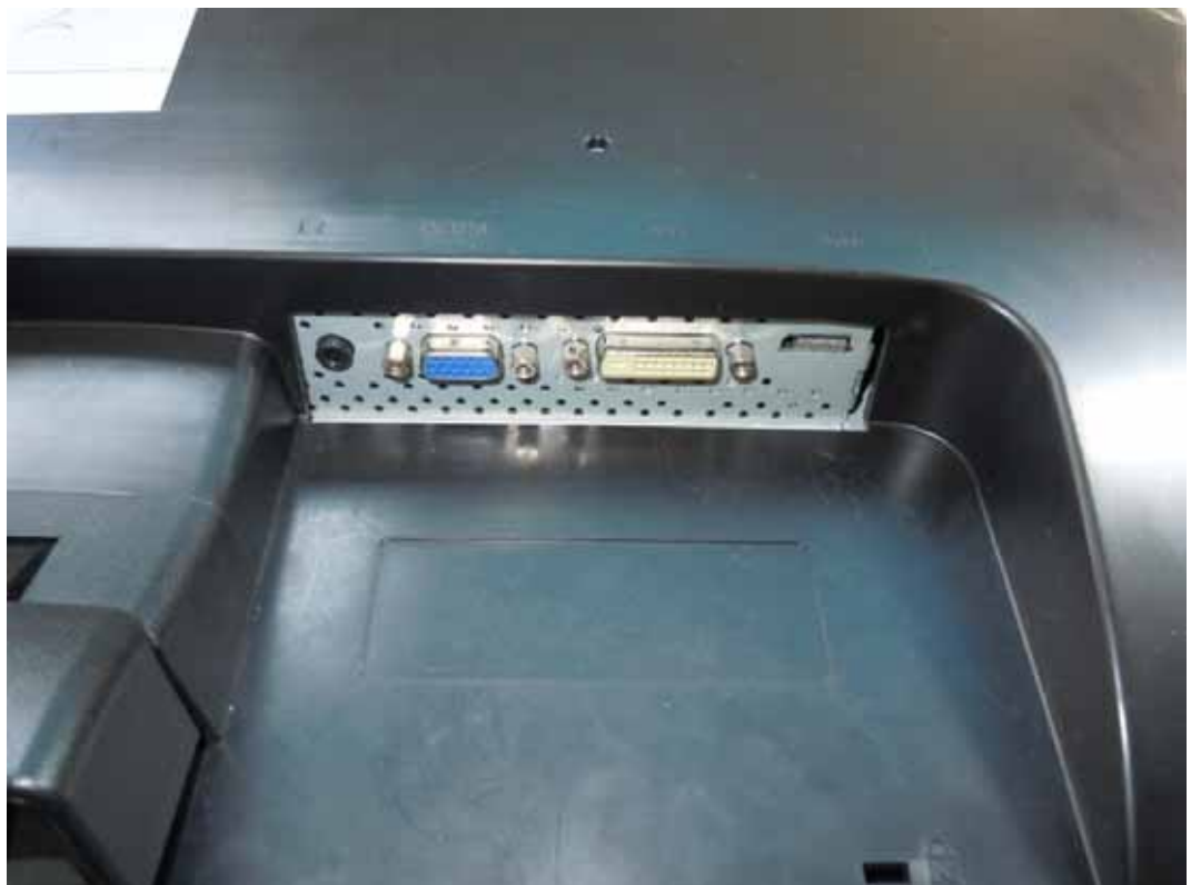
FIGURE 4 LCD MONITOR (M/N: E2541VX) SIGNAL PORTS
