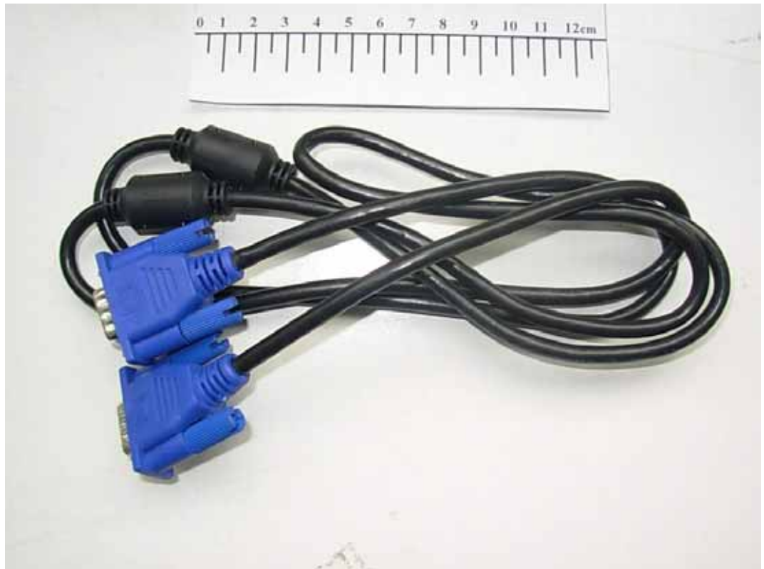
FIGURE 5 LCD MONITOR (M/N: E2541VX) D-SUB CABLE #1
