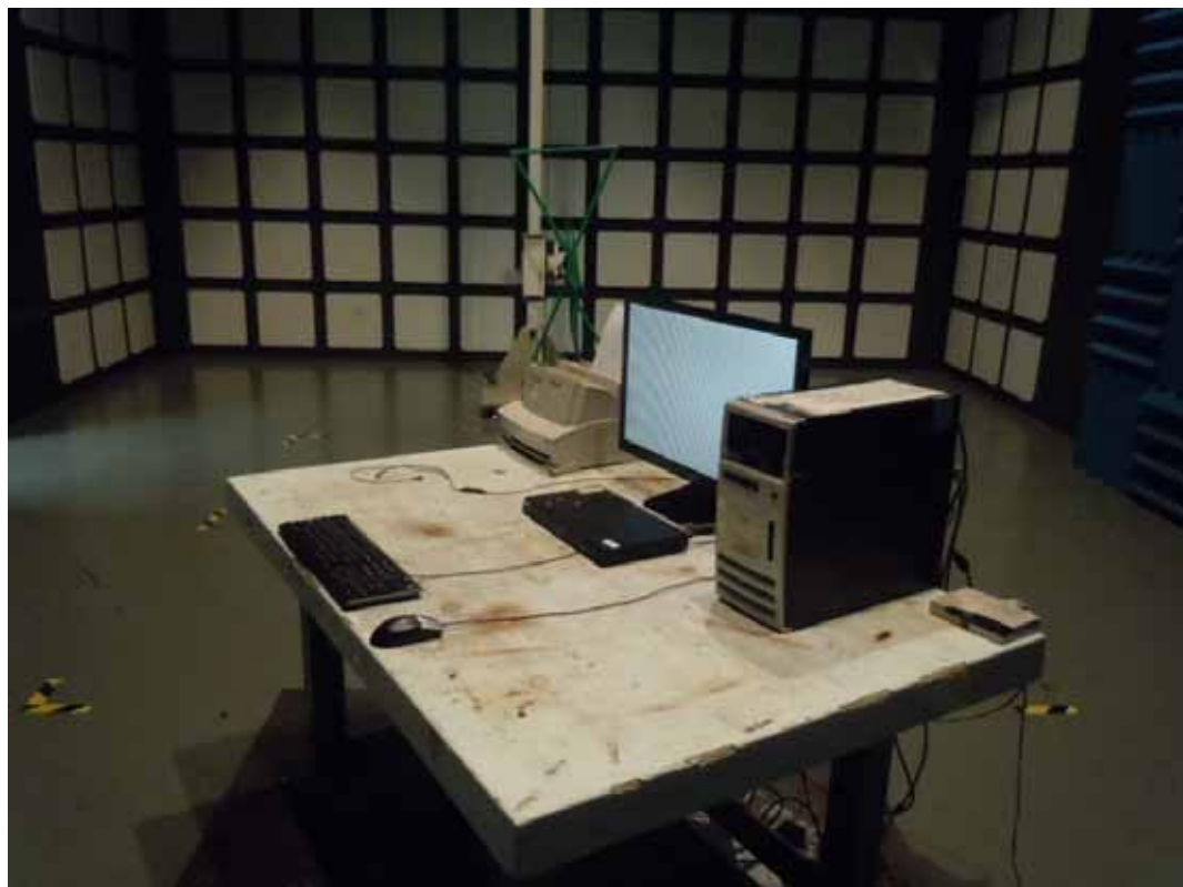
SETUP WITH MAXIMUM DETECTED EMISSION AT VERTICAL POLARIZATION (TEST MODE: DVI 1920*1080@60Hz)
