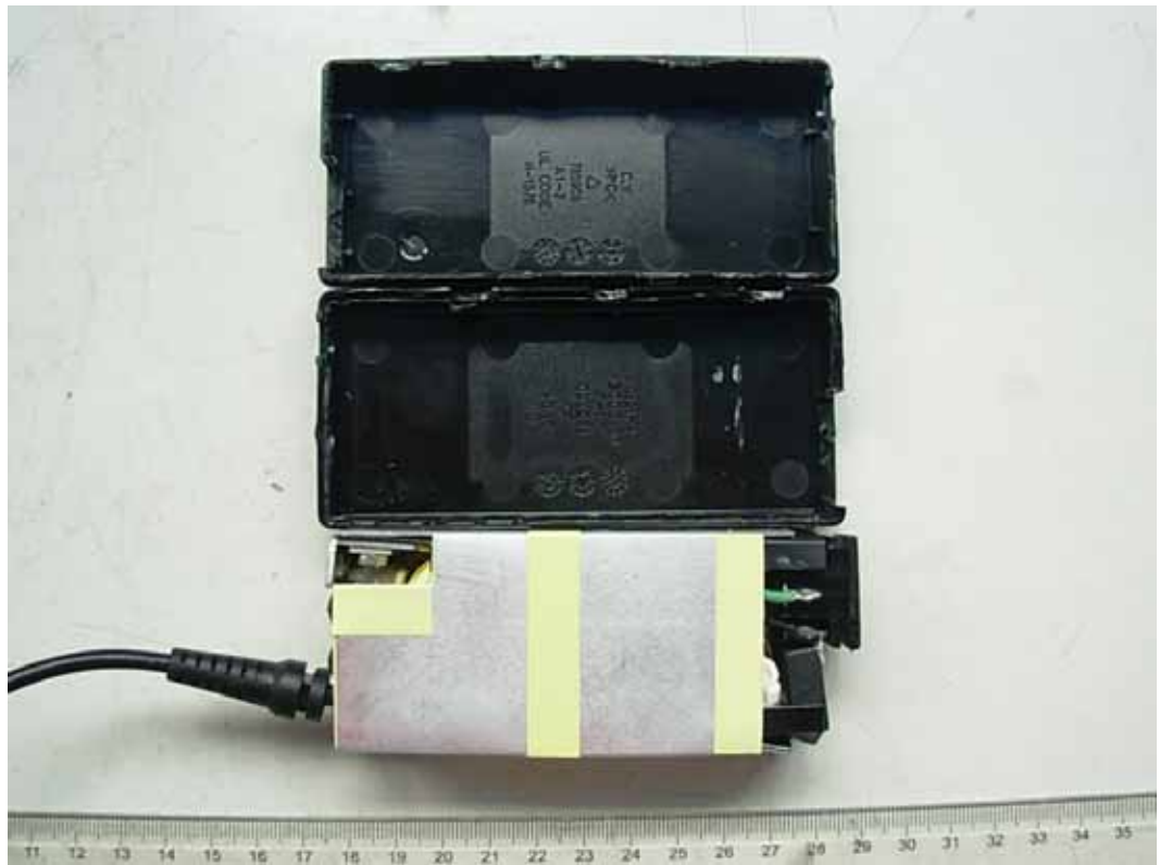
FIGURE 12 LCD MONITOR (M/N: E2750VV) ADAPTER (COVER REMOVED)
