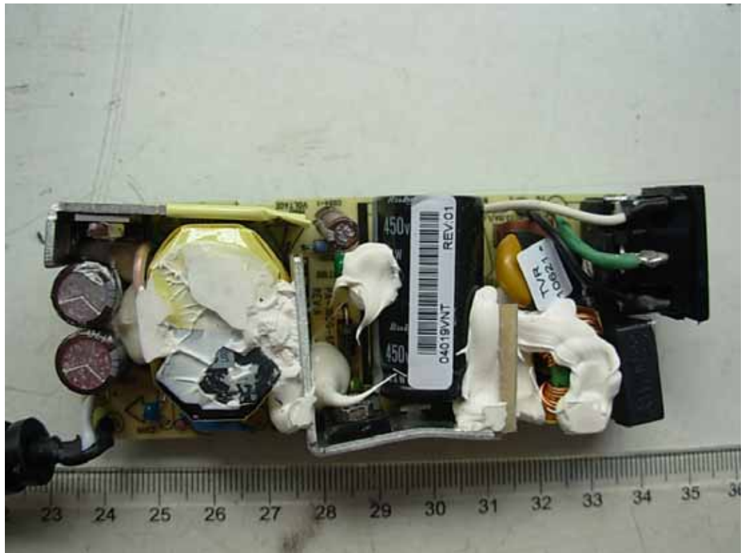
FIGURE 13 LCD MONITOR (M/N: E2750VV) ADAPTER (MAIN BOARD – COMPONENT SIDE)
