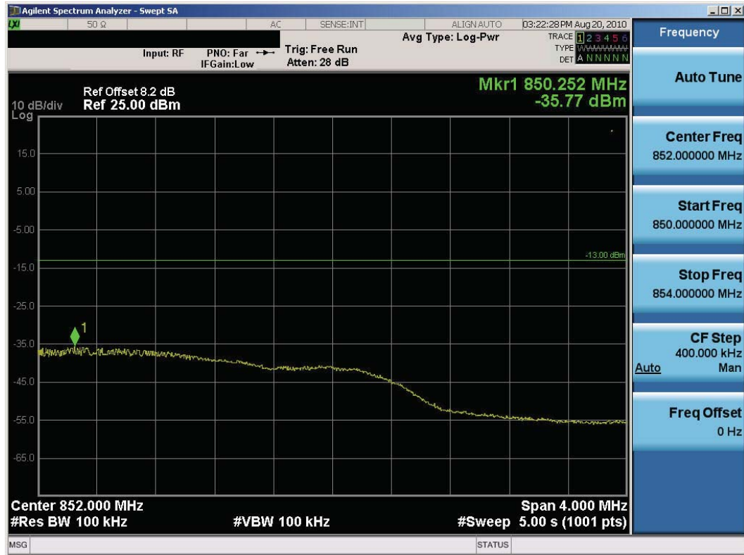
Plot 7-33. 4MHz Span Plot (Cellular WCDMA Mode – Ch. 4233)
