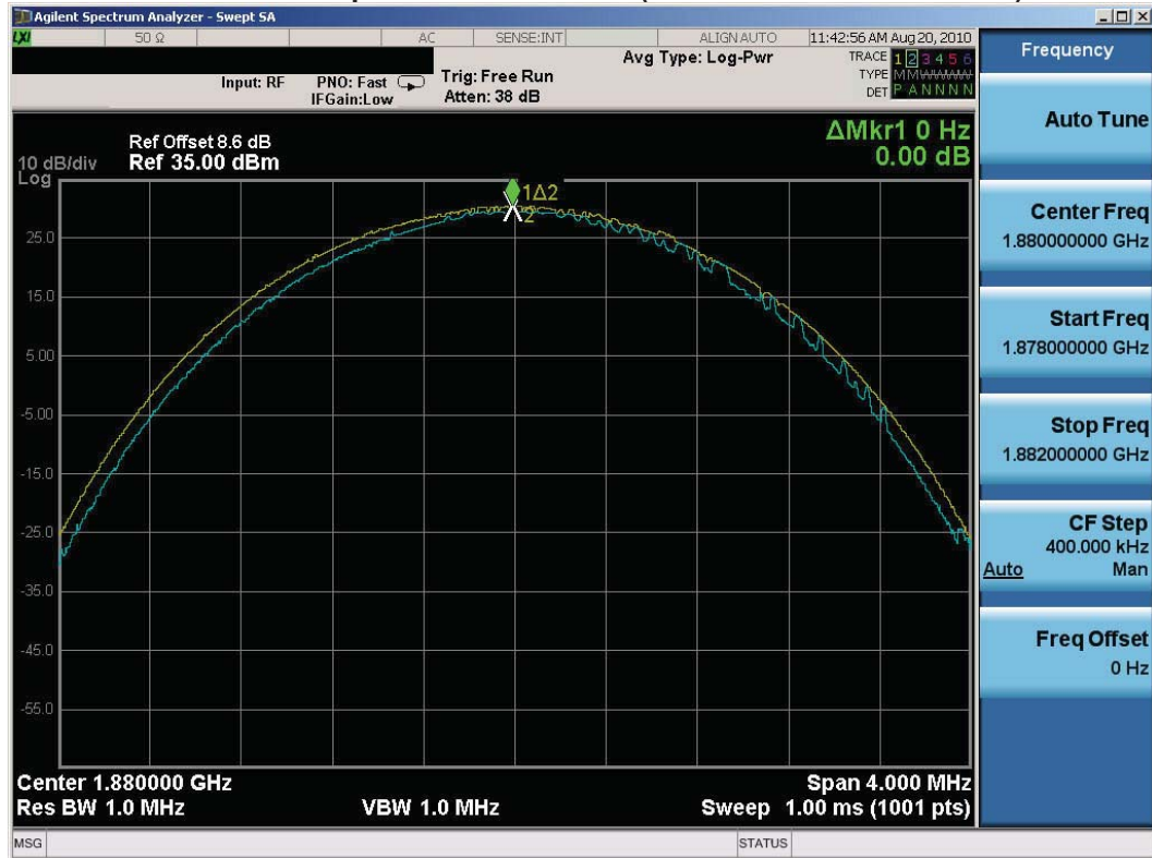
Plot 7-22. Peak-Average Ratio Plot (EDGE1900 Mode – Ch. 661)
