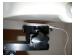
Figure 14.5 Body SAR Test Setup -- w/o Belt-clip --
