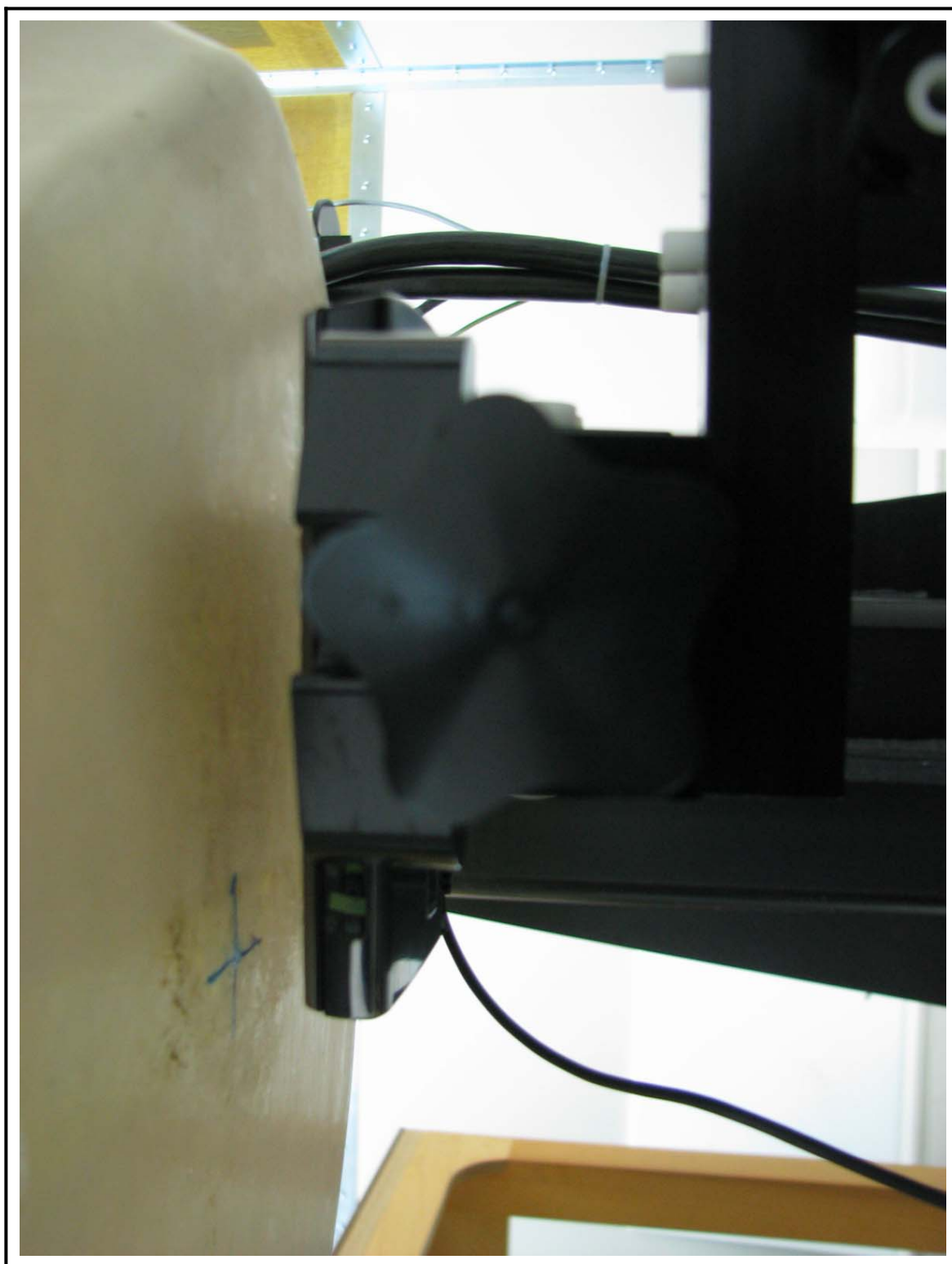
Figure 9 Body SAR Test Setup – w/o Holster
