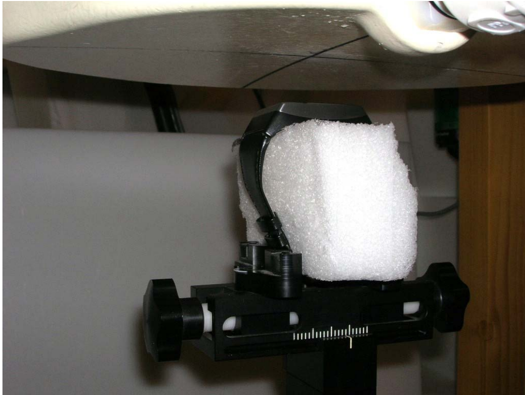
Figure 1 Head/Face SAR Setup (Speakerphone Voice Mode), 1.0 cm spacing
