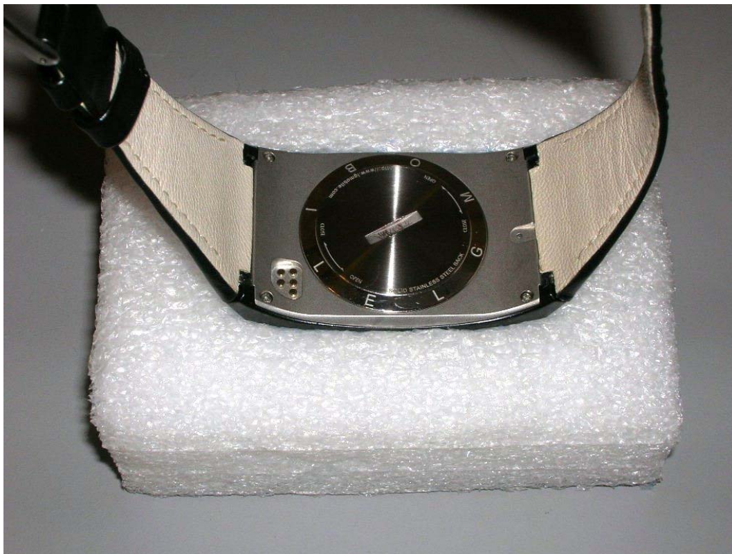
Figure 4 Wrist SAR Setup (Styrofoam holder)
