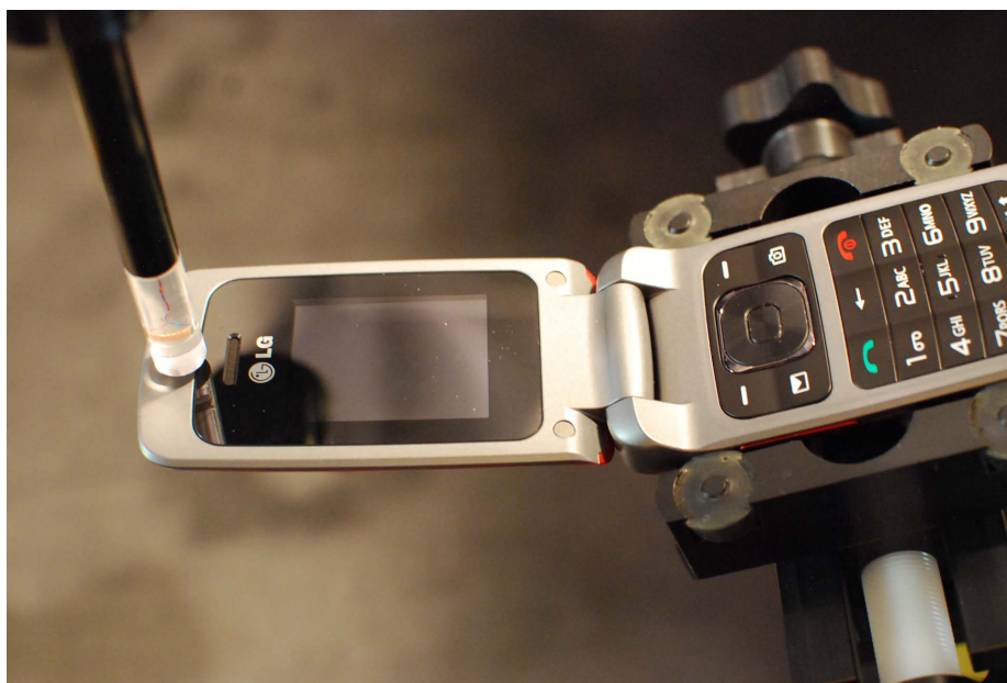
Figure 12-2 Test Setup for Wireless Device
