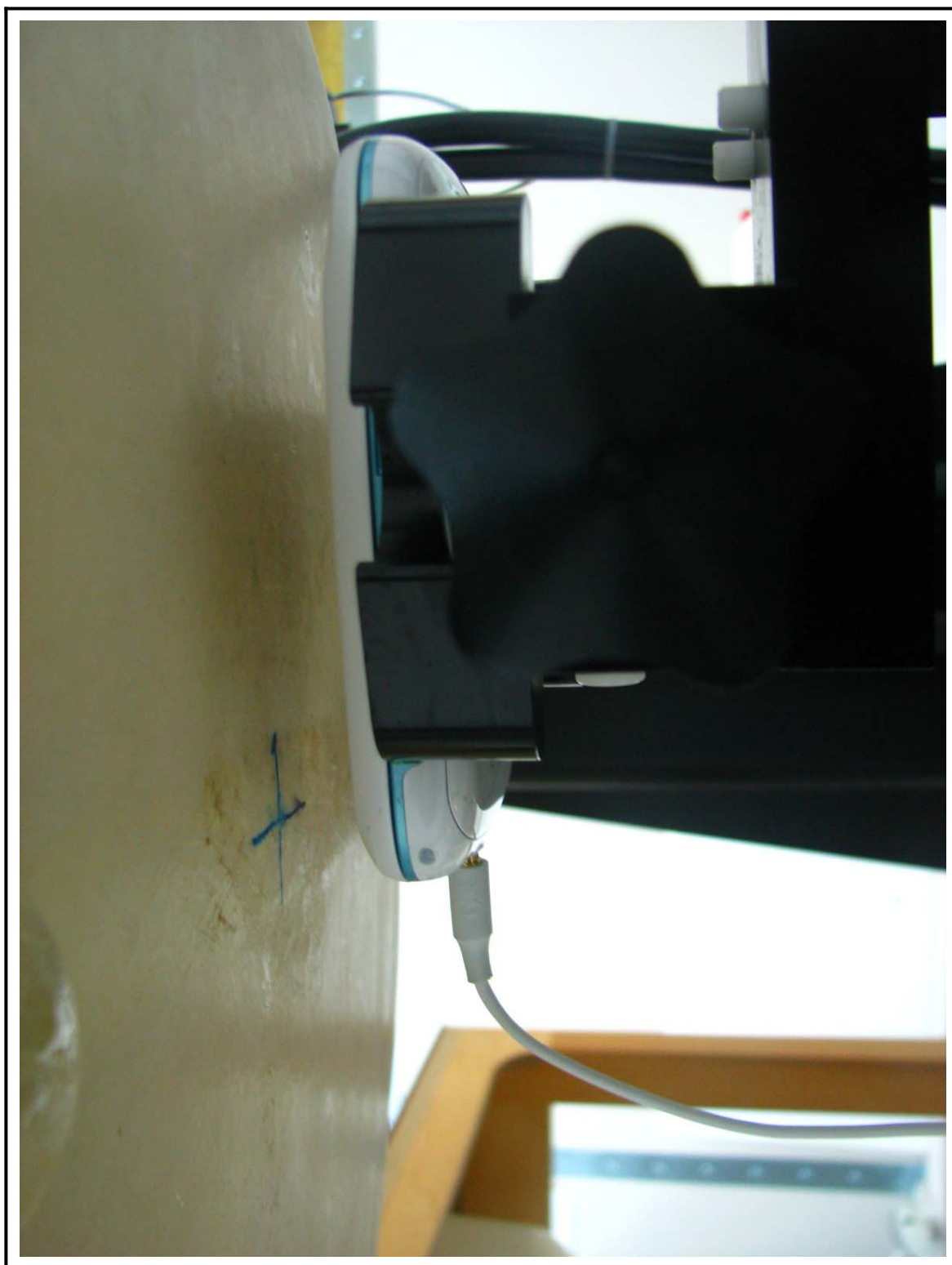
Figure 5 Body SAR Test Setup – w/o Holster
