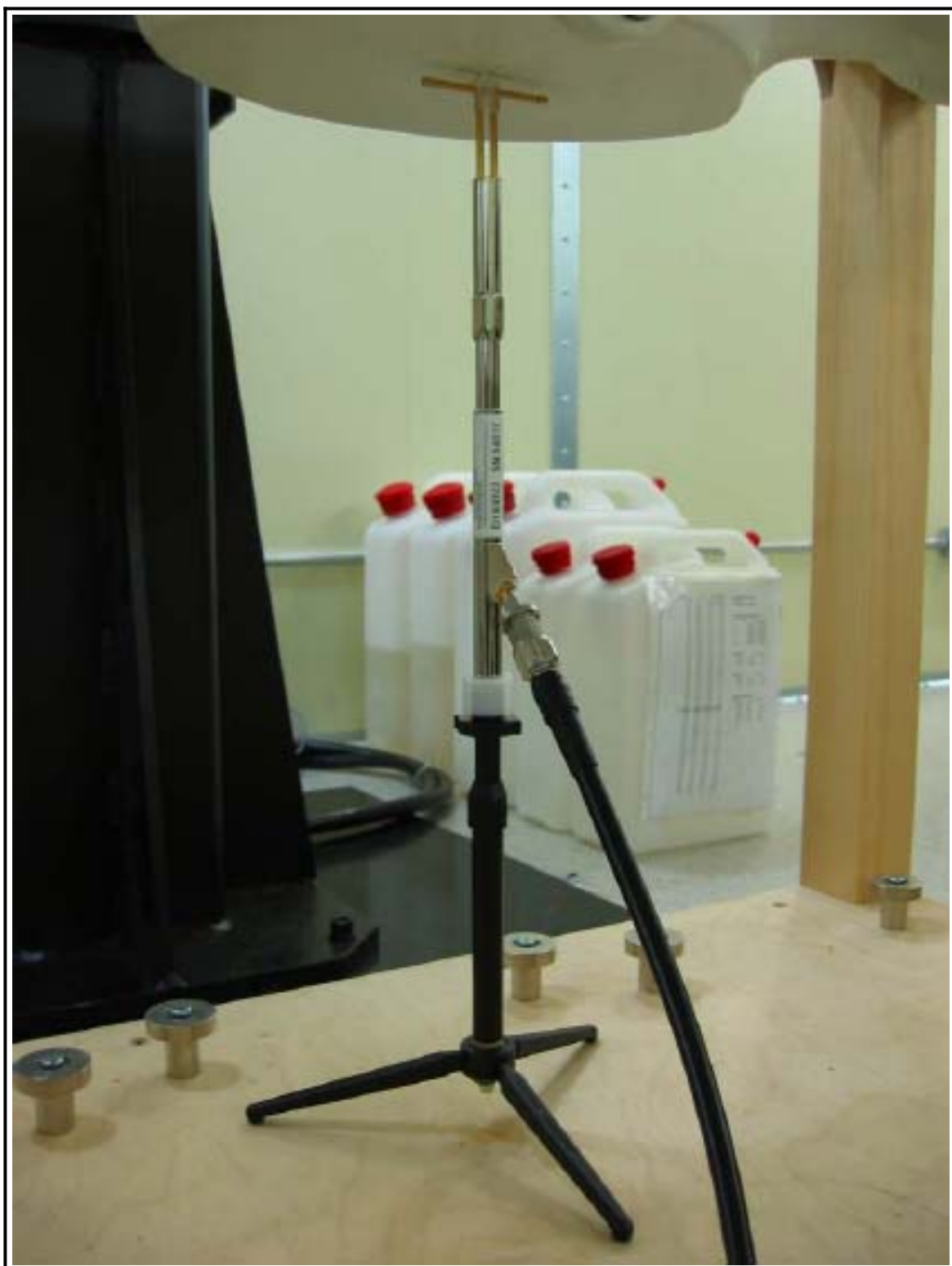
Figure 2 1900 MHz Dipole Validation Test Setup
