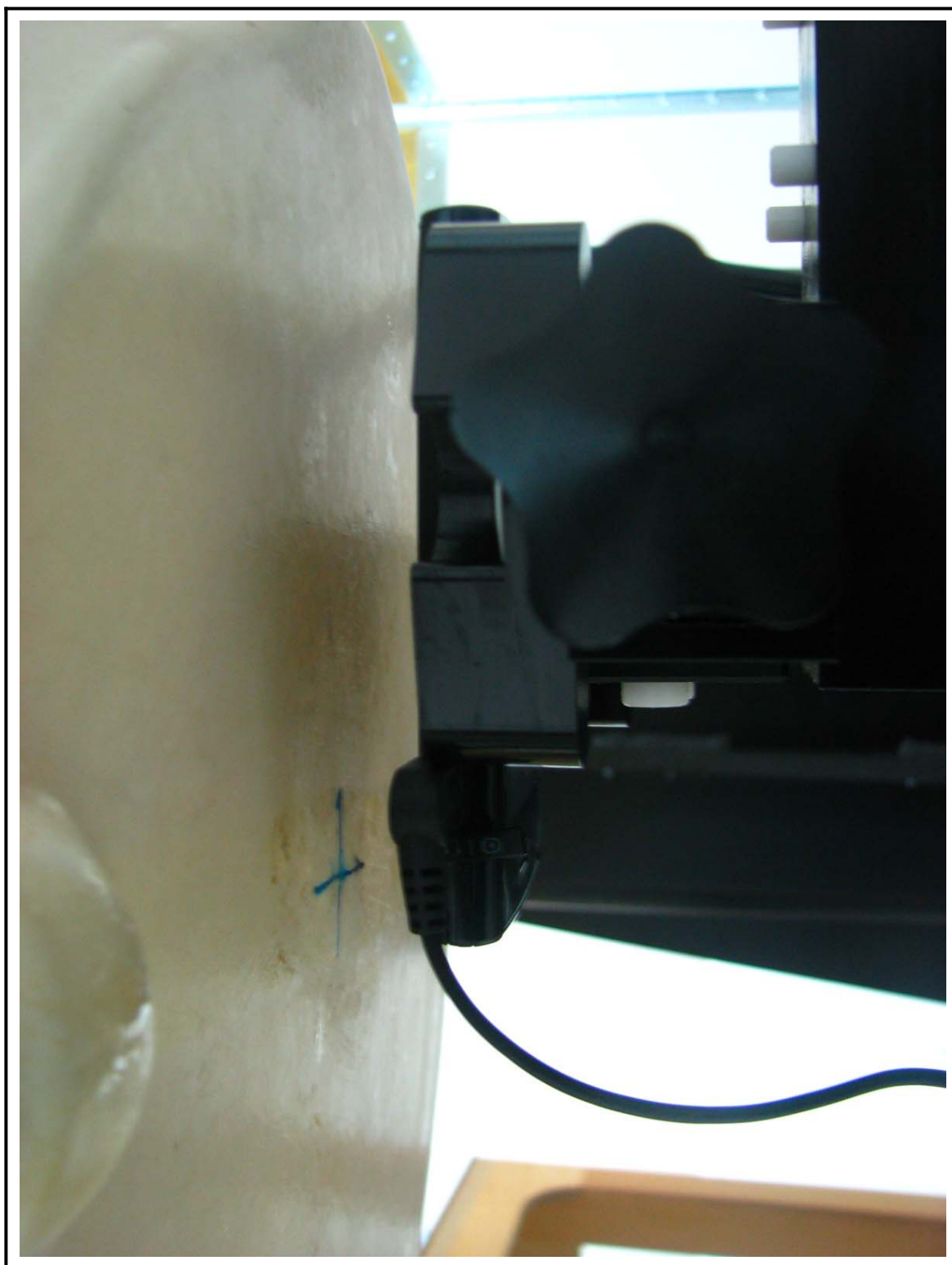
Figure 6 Body SAR Test Setup – w/o Holster
