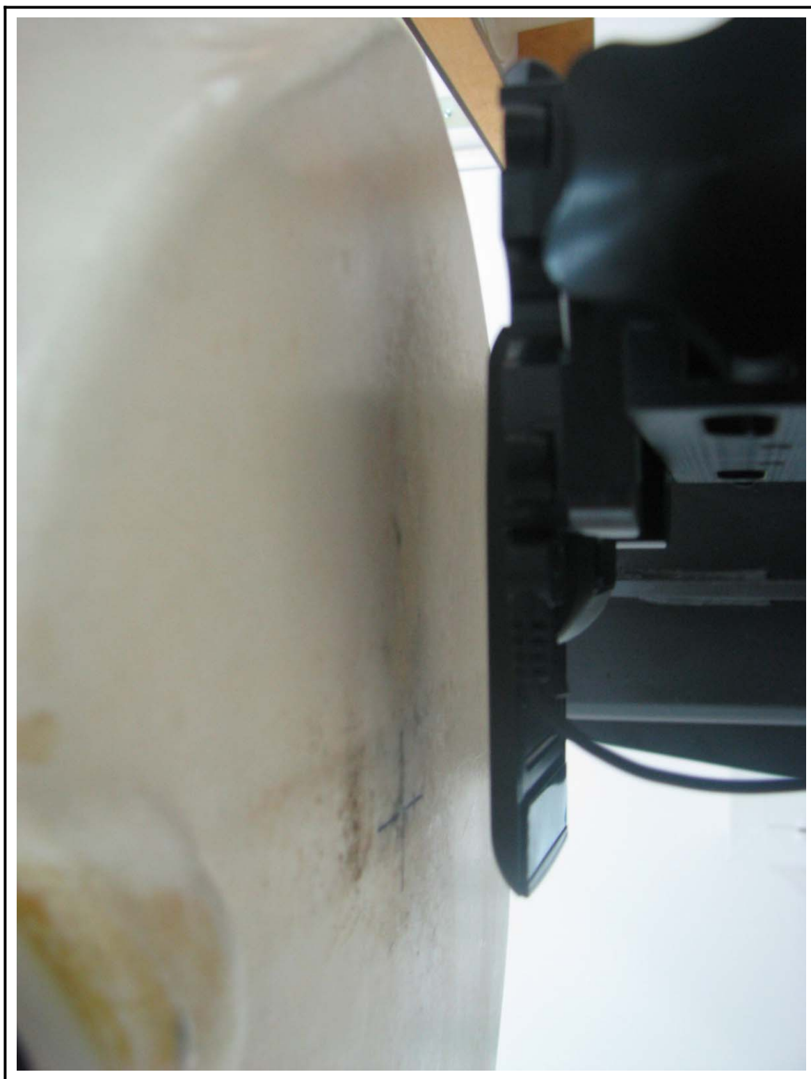
Figure 10 Body SAR Test Setup – w/o Holster
