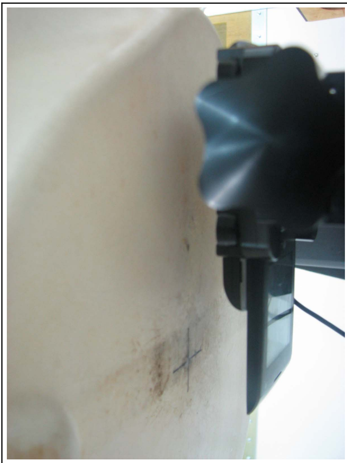
Figure 12 Body SAR Test Setup – w/o Holster
