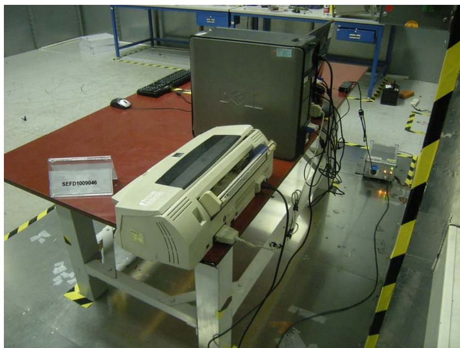
Back View of Conducted Emission Test
