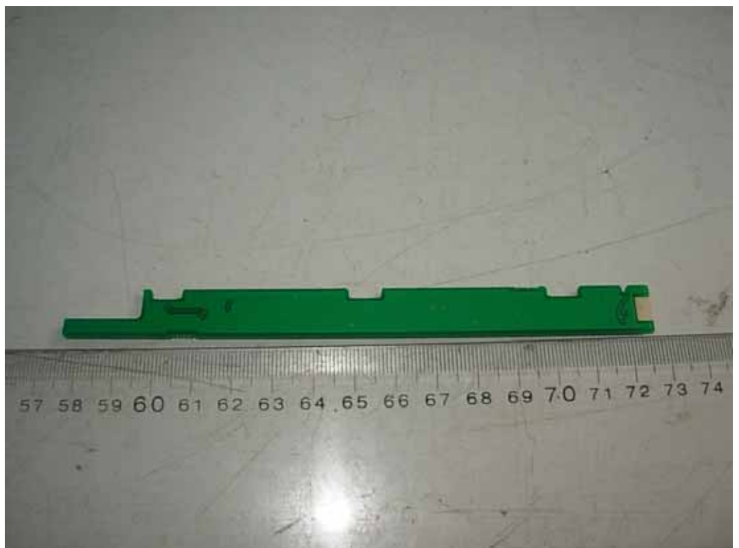
FIGURE 10 LCD MONITOR (M/N: IPS225VX) KEY BOARD (SOLDERED SIDE)
