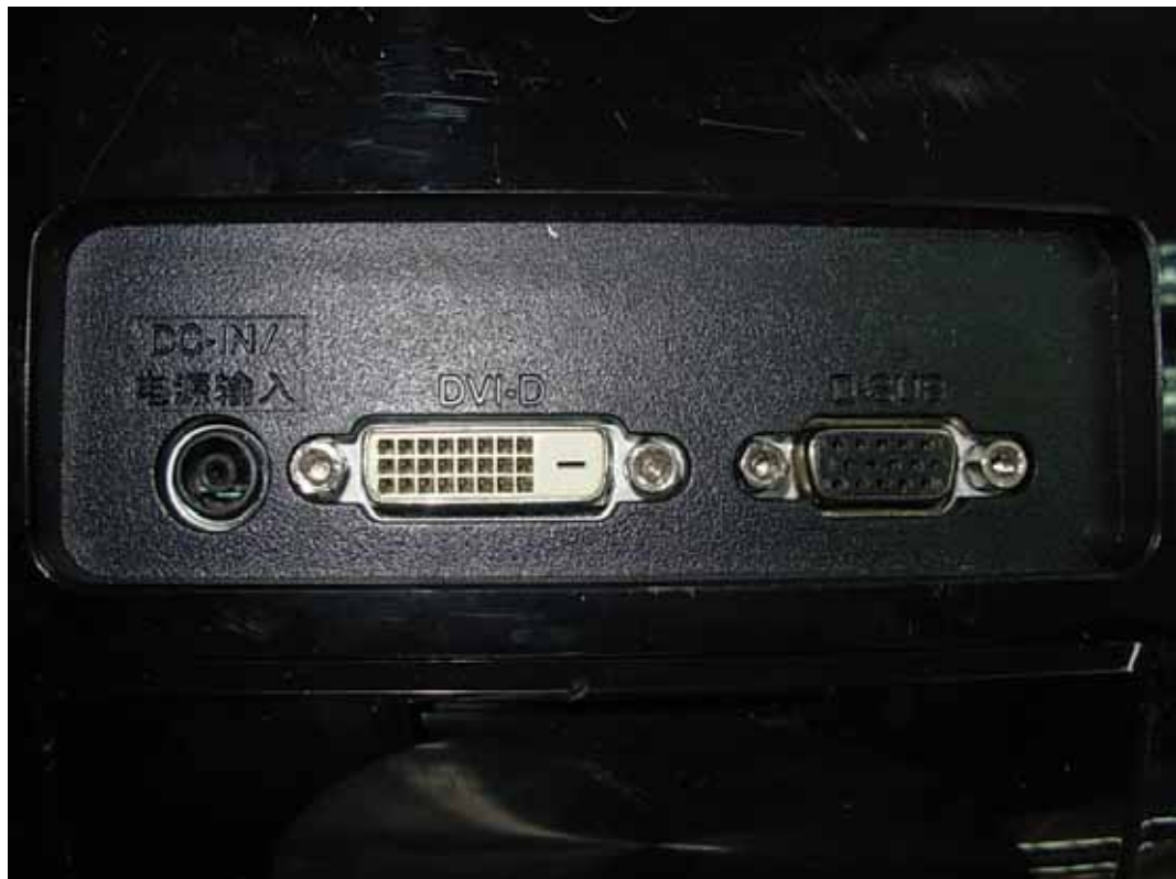
FIGURE 3 LCD MONITOR (M/N: IPS226TX) AC POWER & SIGNAL PORTS
