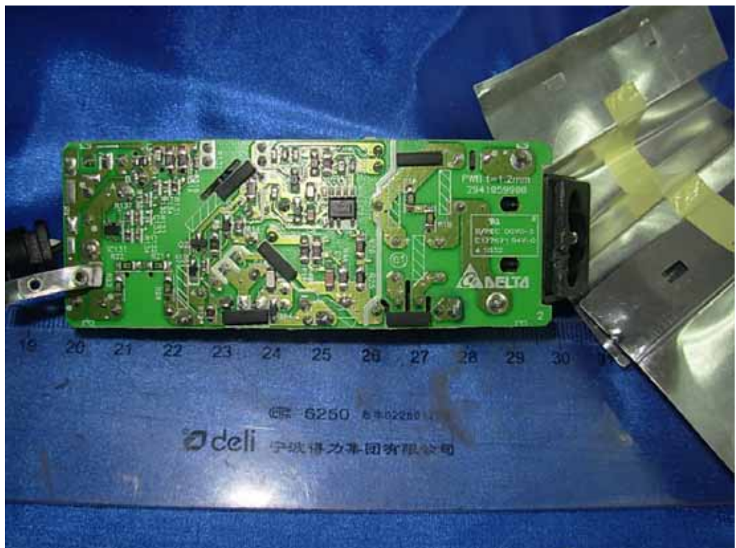
FIGURE 23 LCD MONITOR (M/N: IPS226TX) ADAPTER #2 (MAIN BOARD – SOLDERED SIDE)
