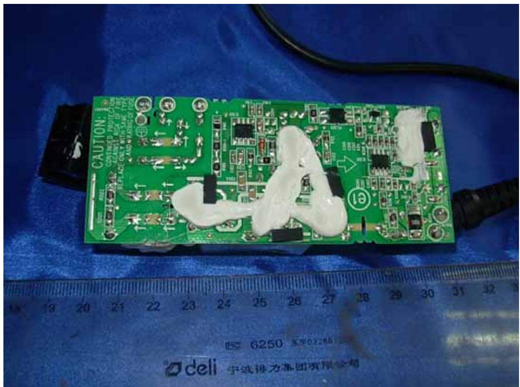
FIGURE 16 LCD MONITOR (M/N: IPS226TX) ADAPTER #1 (MAIN BOARD – SOLDERED SIDE)
