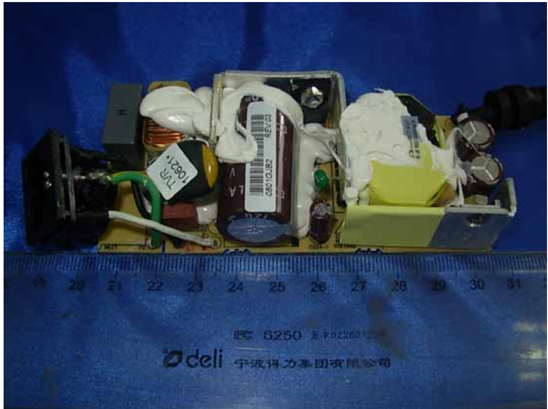
FIGURE 15 LCD MONITOR (M/N: IPS226TX) ADAPTER #1 (MAIN BOARD – COMPONENT SIDE)
