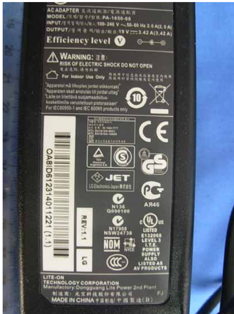
FIGURE 12 LCD MONITOR (M/N: IPS226TX) ADAPTER #1 (LABEL)
