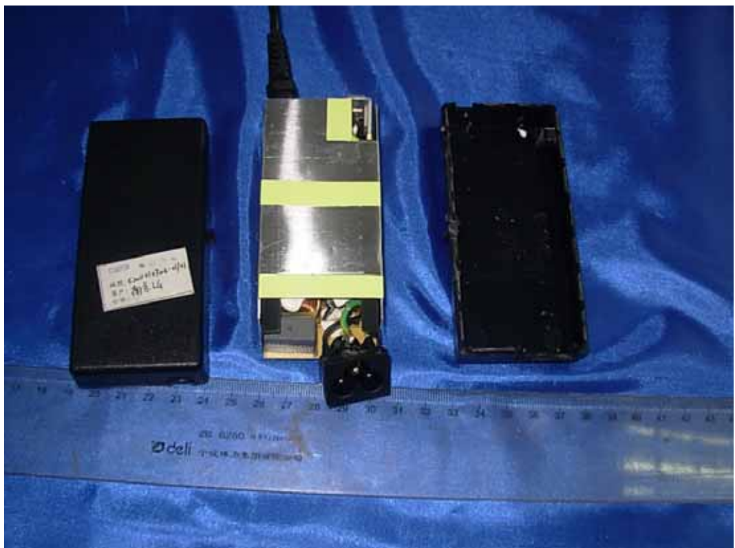
FIGURE 14 LCD MONITOR (M/N: IPS226TX) ADAPTER #1 (COVER REMOVED)
