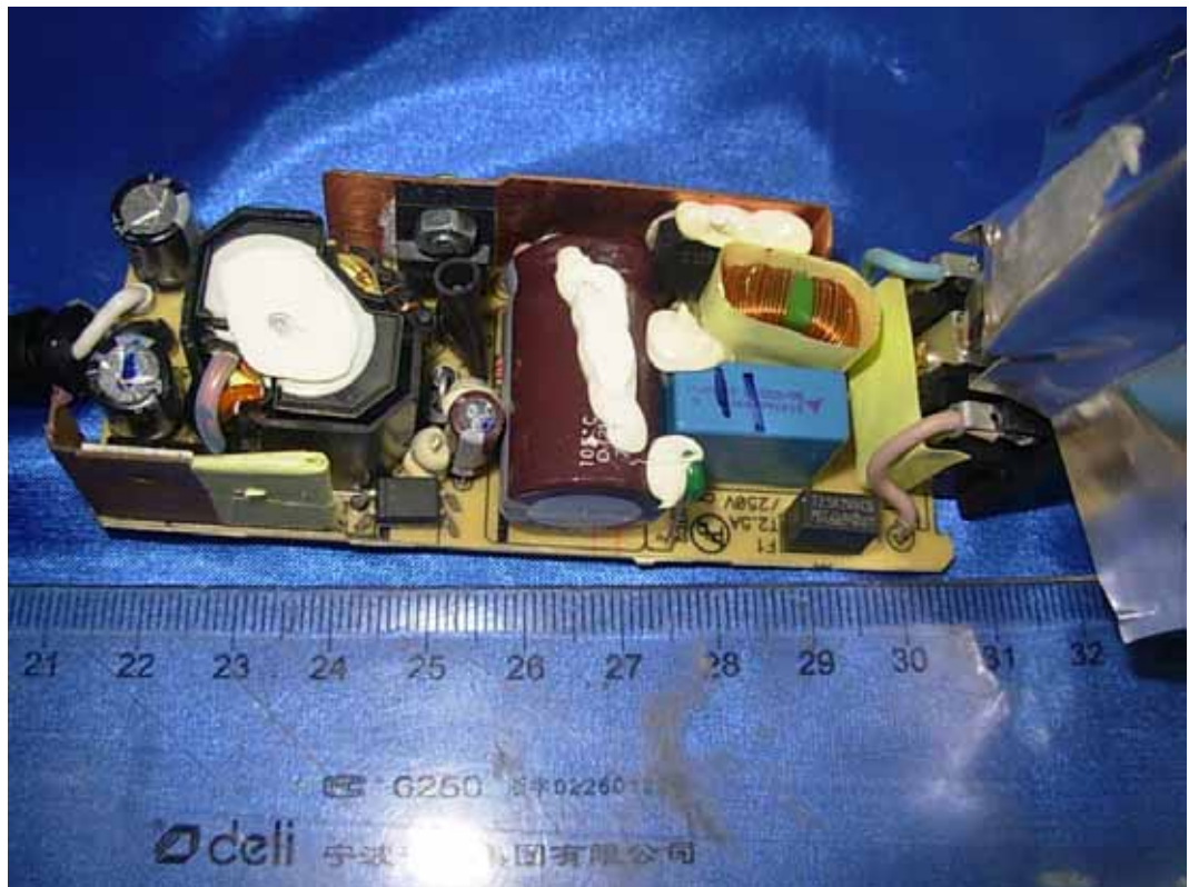
FIGURE 22 LCD MONITOR (M/N: IPS226TX) ADAPTER #2 (MAIN BOARD – COMPONENT SIDE)
