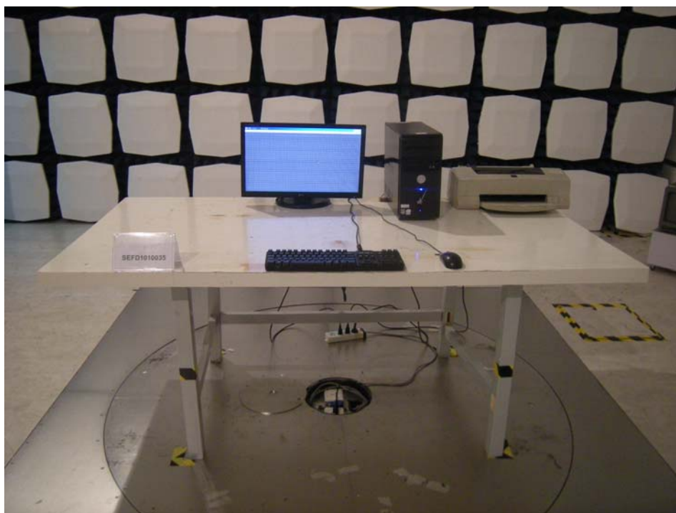
Front View of Radiated Emission Test
