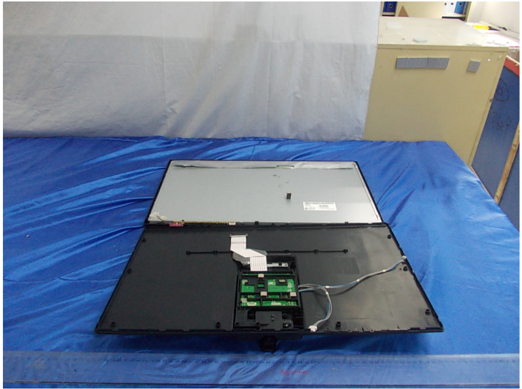
FIGURE 1 LCD MONITOR (M/N: IPS234VA) COVER REMOVED
