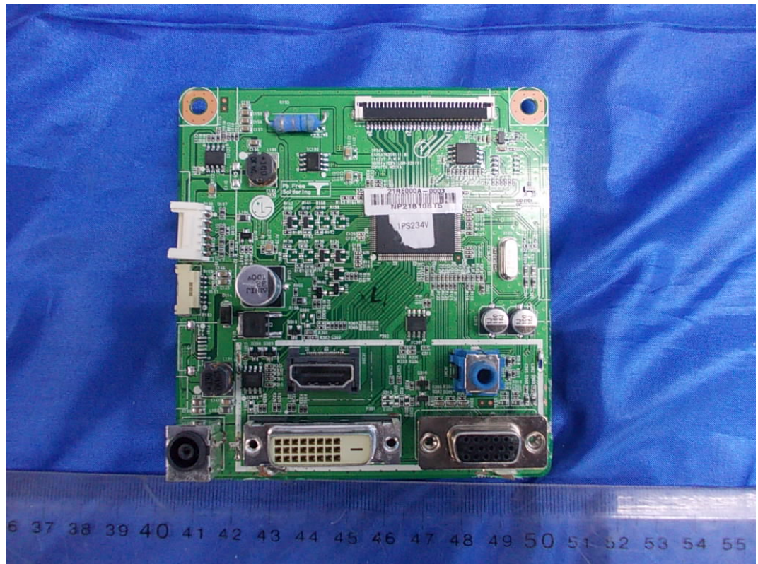
FIGURE 3 LCD MONITOR (M/N: IPS234VA) MAIN BOARD (COMPONENT SIDE)
