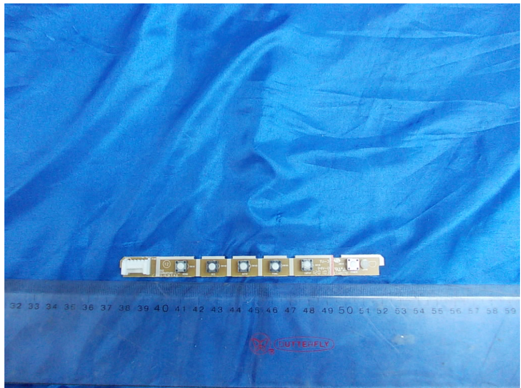
FIGURE 6 LCD MONITOR (M/N: IPS234VA) KEY BOARD (COMPONENT SIDE)
