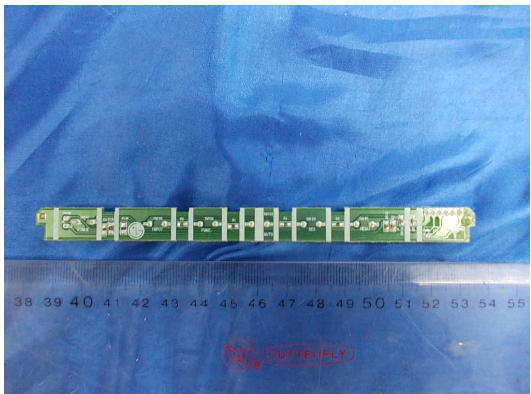
FIGURE 7 LCD MONITOR (M/N: IPS234VA) KEY BOARD (SOLDERED SIDE)
