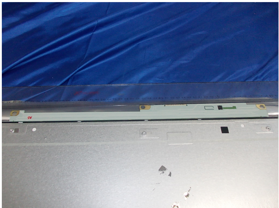
FIGURE 9 LCD MONITOR (M/N: IPS234VA) LCD PANEL BOARD (SOLDERED SIDE)
