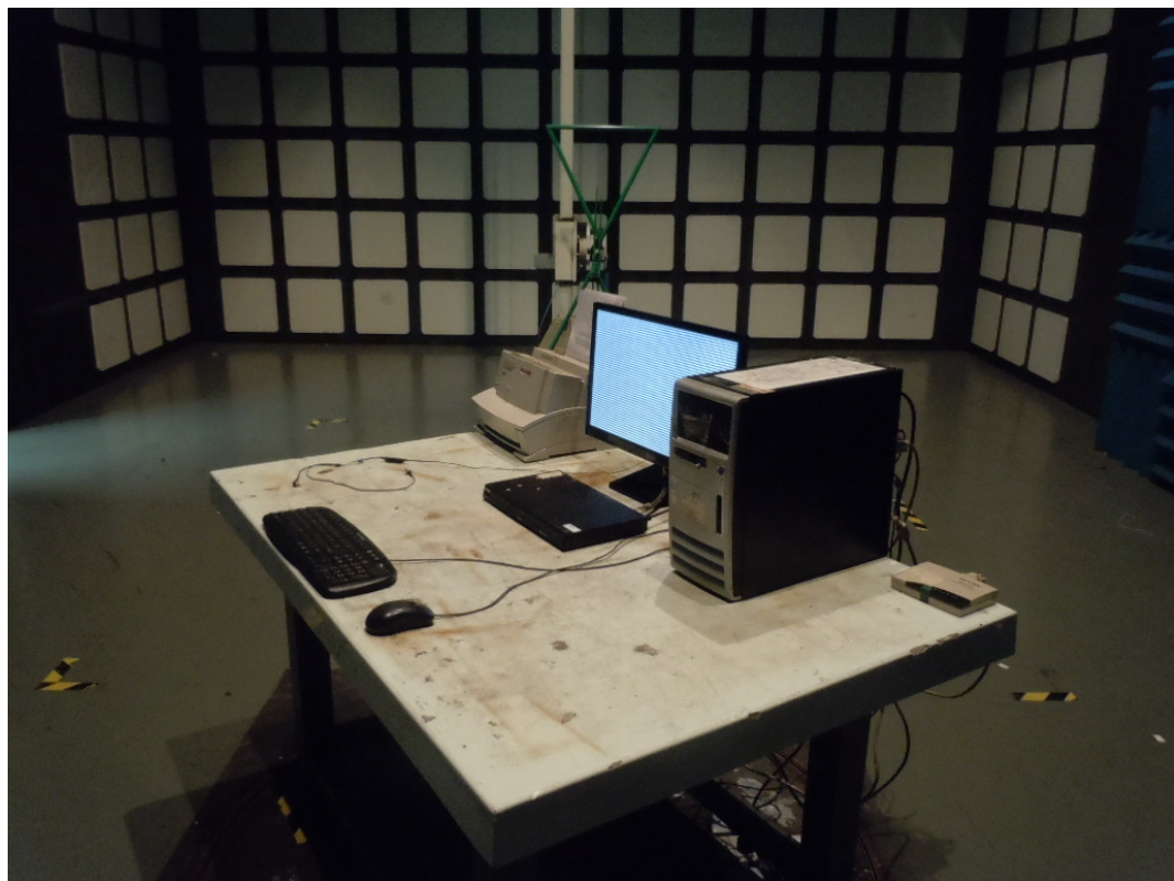
SETUP WITH MAXIMUM DETECTED EMISSION AT VERTICAL POLARIZATION (TEST MODE: DVI 1920*1080@60Hz ADAPTER #1)
