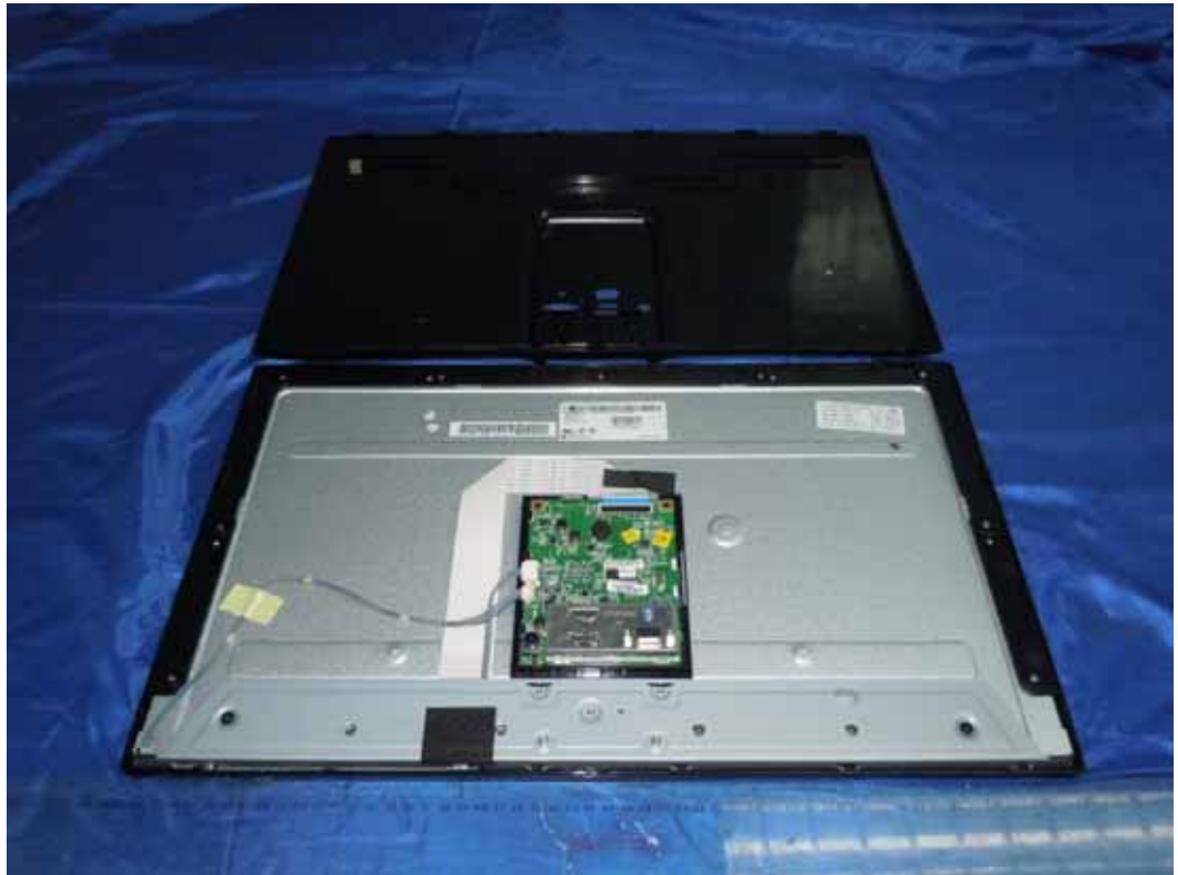
FIGURE 1 LCD MONITOR (M/N: IPS237LY) COVER REMOVED
