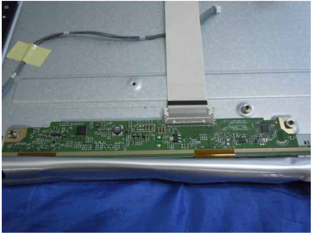
FIGURE 9 LCD MONITOR (M/N: IPS237LY) LCD PANEL BOARD (COMPONENT SIDE-1)
