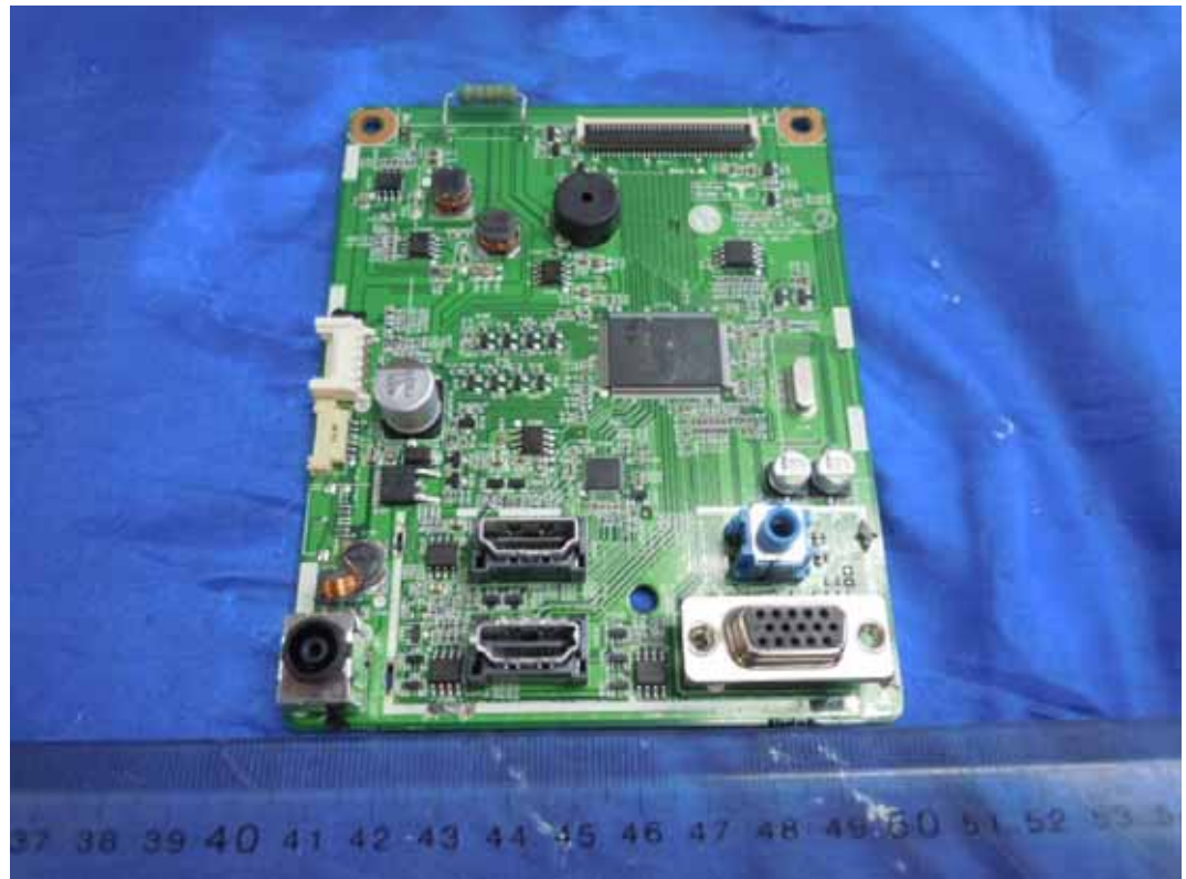
FIGURE 3 LCD MONITOR (M/N: IPS237LY) MAIN BOARD (COMPONENT SIDE)
