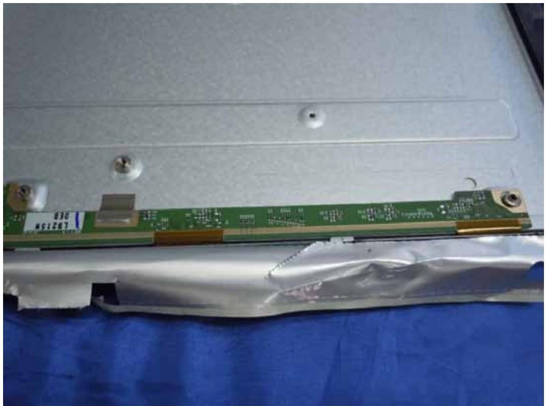
FIGURE 10 LCD MONITOR (M/N: IPS237LY) LCD PANEL BOARD (COMPONENT SIDE-2)
