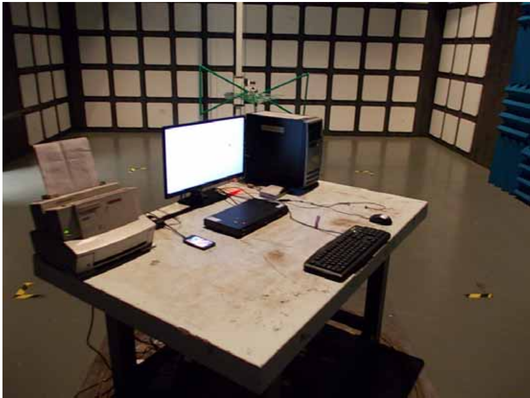
SETUP WITH MAXIMUM DETECTED EMISSION AT HORIZONTAL POLARIZATION (TEST MODE: HDMI 1920*1080@60Hz Adapter #1)
