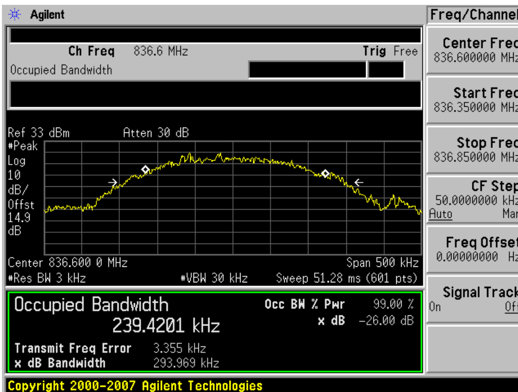
Plot 7-10. Occupied Bandwidth Plot (EDGE850 Mode – Ch. 190)
