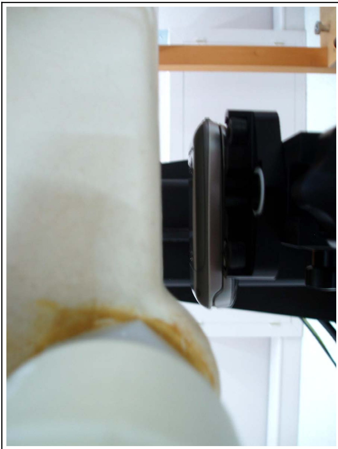
Figure 15 Body SAR Test Setup – w/o Holster
