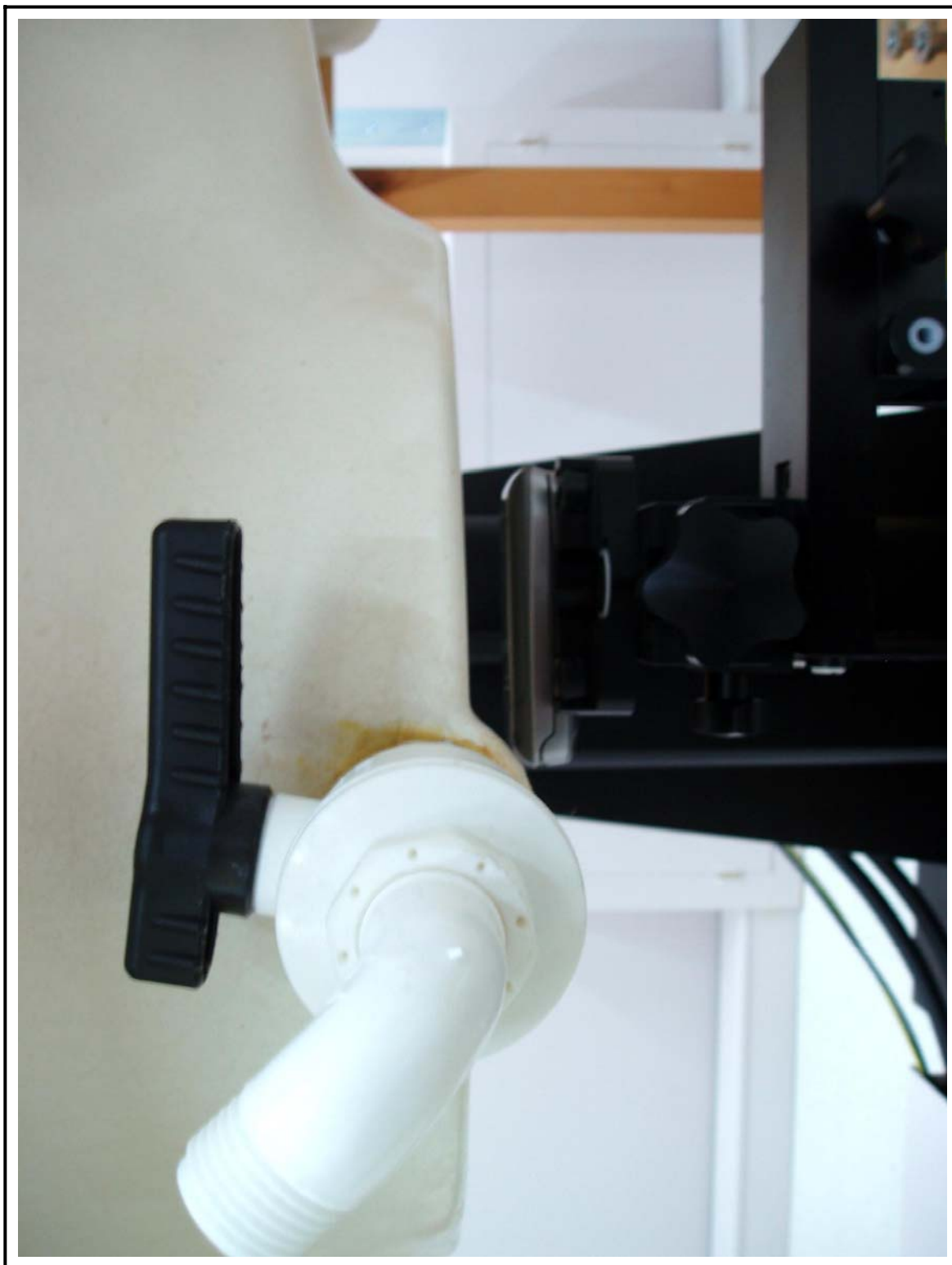
Figure 14 Body SAR Test Setup – w/o Holster
