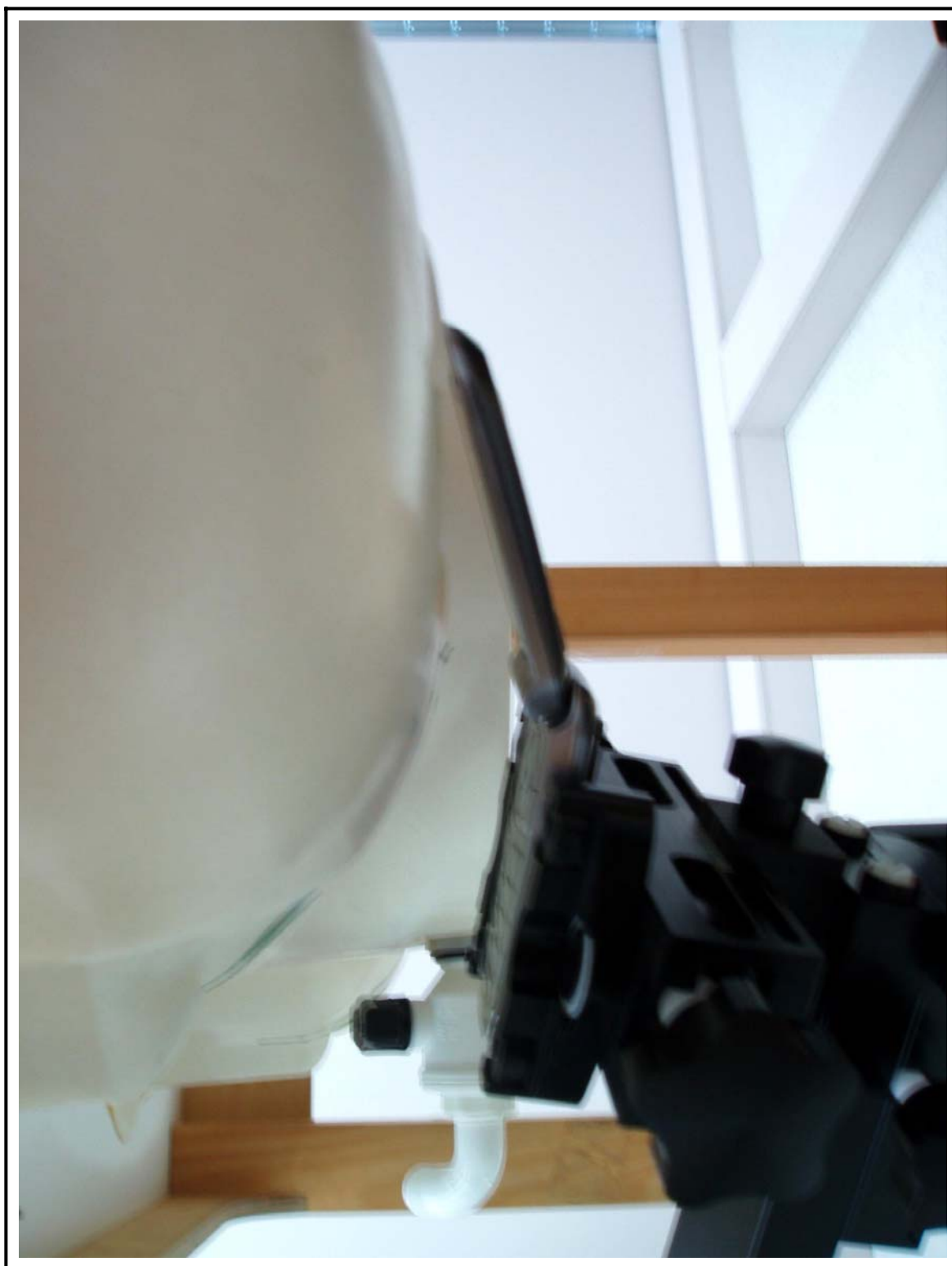
Figure 12 Left Head SAR Test Setup - Ear Tilt Position
